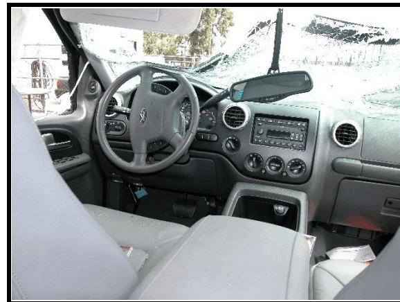
Figure 12. Non-deployed driver's air bag
