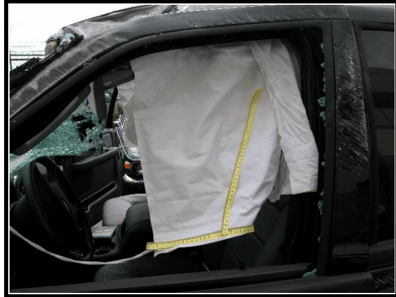
Figure 11. Exterior view of left side curtain
