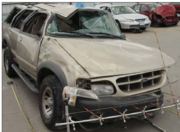
Figure 14: Front right view of rollover damage to case vehicle
