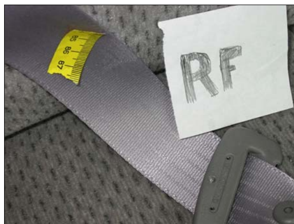
Figure 13: Case vehicle's front right safety belt showing friction burns (indicated by yellow tape) on webbing
