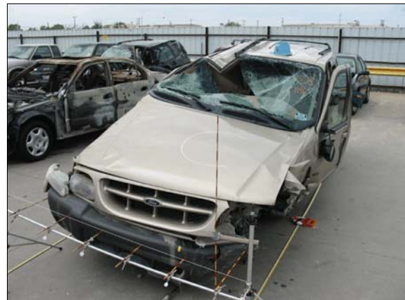
Figure 5: Ford's front left and left fender damage from impact with the case vehicle, and top damage due to the subsequent rollover.
