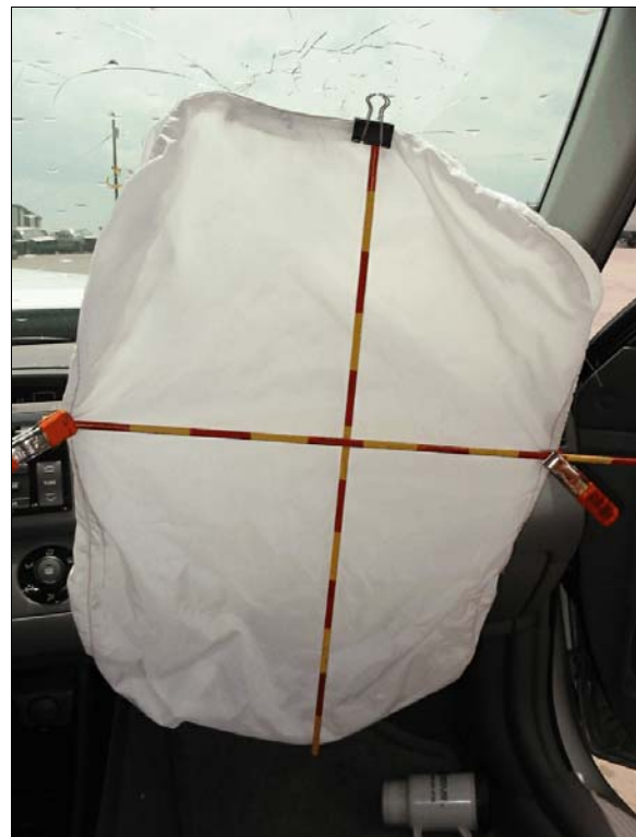
Figure 12: Front surface of case vehicle's deployed front right passenger air bag showing no obvious evidence of occupant contact
