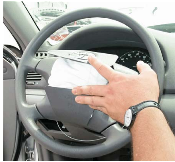
Figure 8: Overview of driver's air bag module cover flaps
