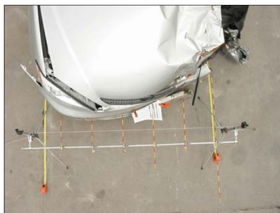
Figure 7: Overhead view of case vehicle’s front crush profile, each increment on rods is 5 cm (2 in)
