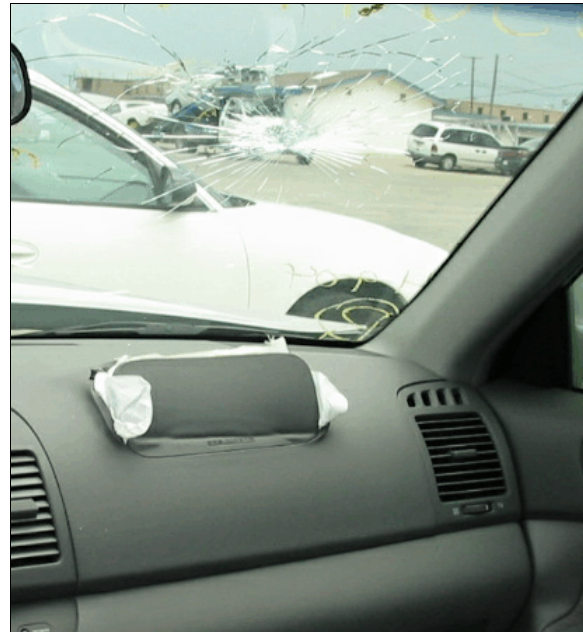
Figure 11: Overview of location of front right air bag, air bag module flap and cracked windshield from deployment
