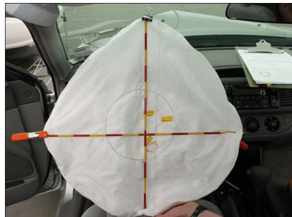
Figure 9: Case vehicle's deployed driver air bag, occupant contact evidence highlighted with yellow tape
