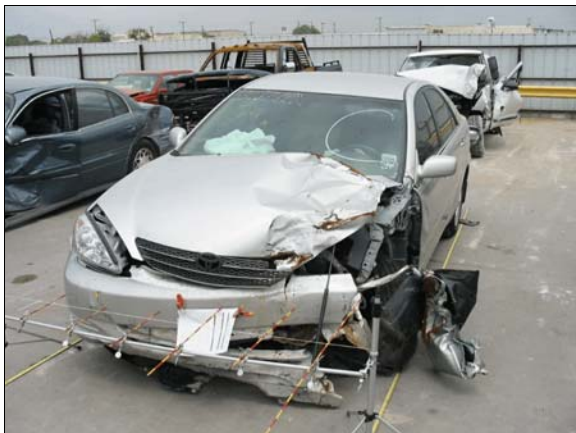
Figure 4: Case vehicle's front left damage and damage to left fender and wheel assembly from the impact with the Ford
