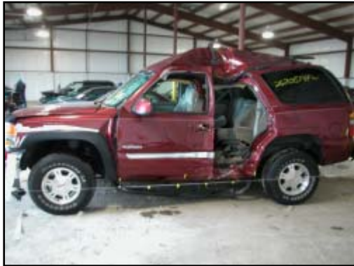
Figure 5. Sill level crush profile.
