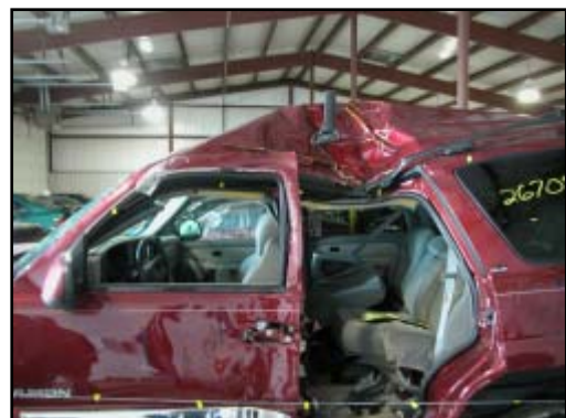
Figure 7. Roof side rail crush profile.
