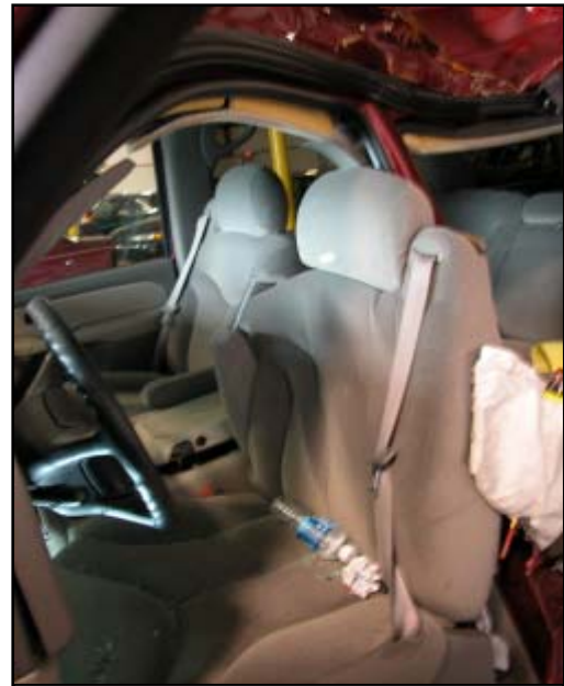
Figure 13. Driver’s integrated 3-point manual lap and shoulder safety belt.
