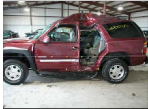
Figure 6. Mid-door crush profile.
