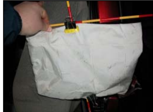
Figure 11. Inboard aspect of driver's side impact air bag.
