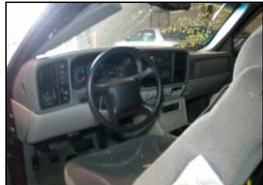
Figure 12. Non-deployed frontal air bag system.
