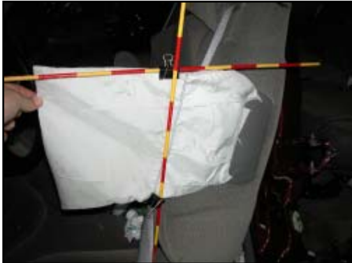
Figure 10. Outboard aspect of driver's side impact air bag.
