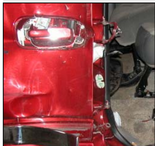
Figure 8. Left rear door B-pillar mounted hinges. Torn during utility pole impact.
