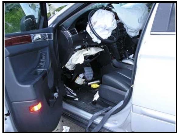
Figure 25. Overview of driver air bag, knee air bag, and passenger frontal air bag
