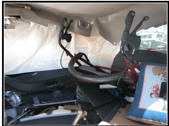
Figure 28. View of air curtain covering third row seat
