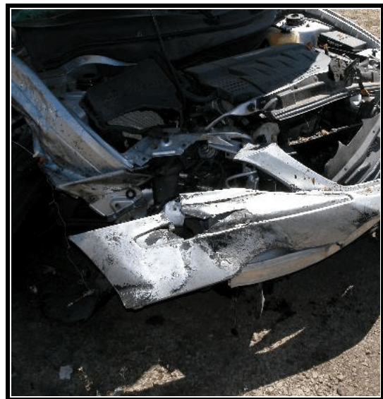
Figure 6. Contact damage from guardrail impact
