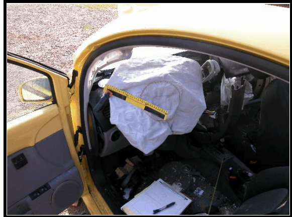
Figure 11. Driver's air bag
