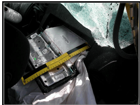
Figure 14. Back side of passenger air bag module cover—showing tether to base of cover
