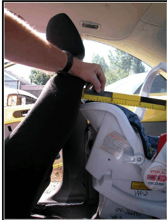
Figure 18. Distance between infant seat and vehicle seat back
