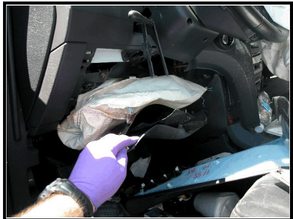
Figure 26. Close up view of knee air bag
