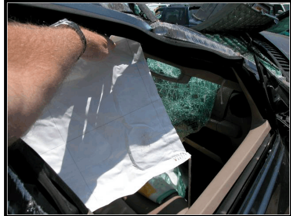
Figure 10. Road abrasions to front right portion of side curtain
