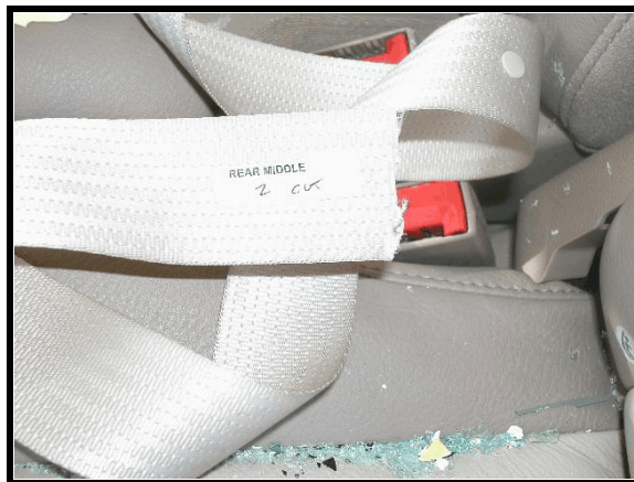
Figure 14. Second row, center, seat belt cut
