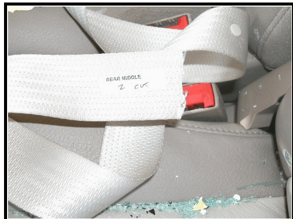
Figure 9. Second row, center, seat belt cut
