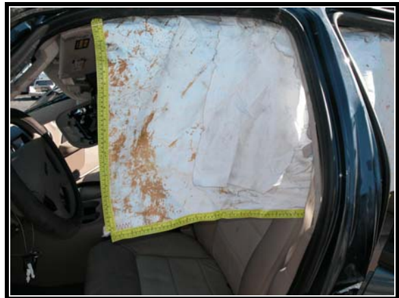
Figure 13. Driver's side curtain - Dirt on bag
