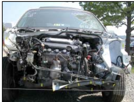
Figure 5. Close-up view of the two crush profiles documented for this impact.
