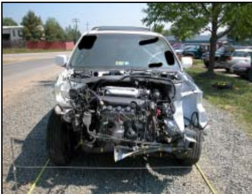
Figure 4. Frontal damage to the 2003 Acura MDX.
