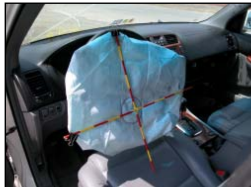
Figure 7. Deployed driver's frontal air bag.
