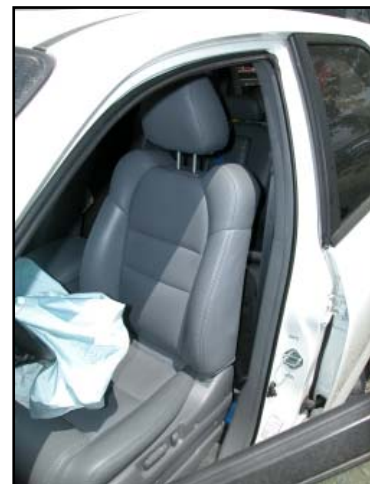
Figure 9. Driver's seat. Note: The safety belt is taut against the B-pillar.
