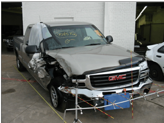
Figure 3: Overview of the damage [each stripe on rods is 5 cm (2 in)] to the right corner of the front bumper, hood, right fender and right front wheel (case photo #21)
