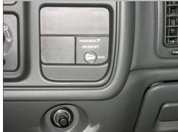
Figure 12: Case vehicle’s front right air bag suppression switch (case photo #39)
