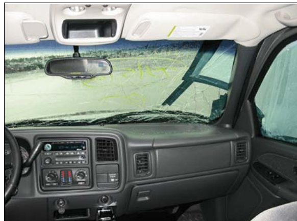
Figure 11: Overview of the right instrument panel and location of front right air bag (case photo #40)
