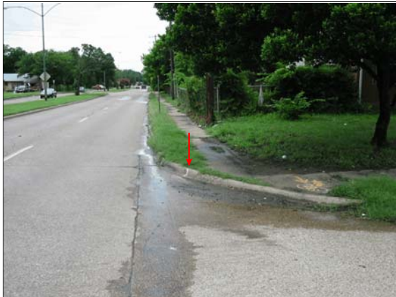
Figure 2: Approach of the case vehicle to impact with the utility pole; Note, arrow shows tire scuff on curb; at white chalk mark, not the broad scuff (case photo #04)
