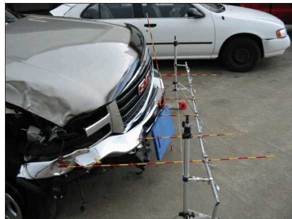
Figure 6: Right side view of crush profile to case vehicle's front bumper prior to adjustment of baseline placement (case photo #20)
