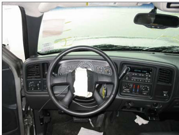
Figure 7: Overview of steering wheel, air bag module flaps and left instrument panel (case photo #28)
