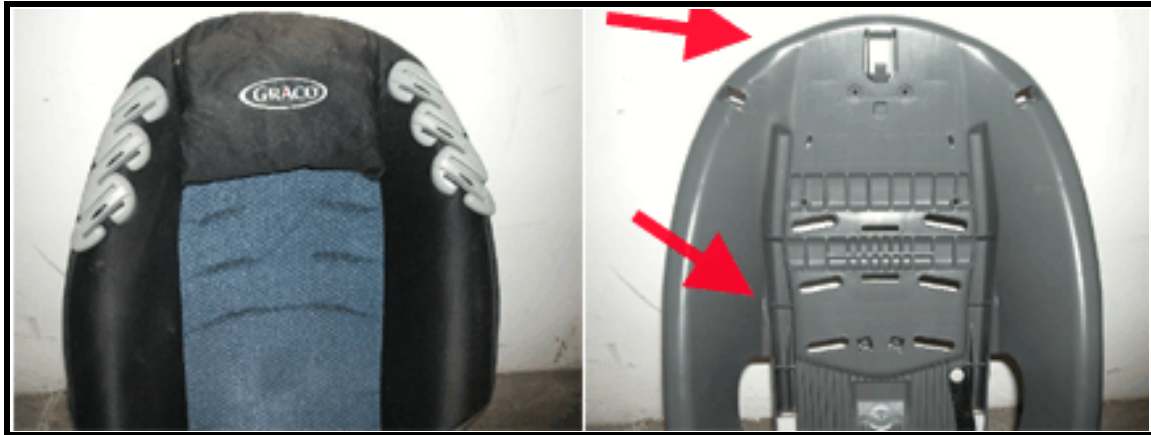
Figure 9. Booster seat with cover on and off. Right image locates stress marks.
