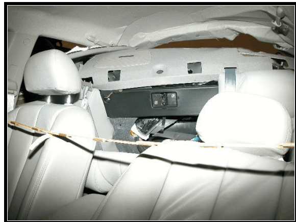
Figure 6. Rear seat intrusion, Nissan Altima
