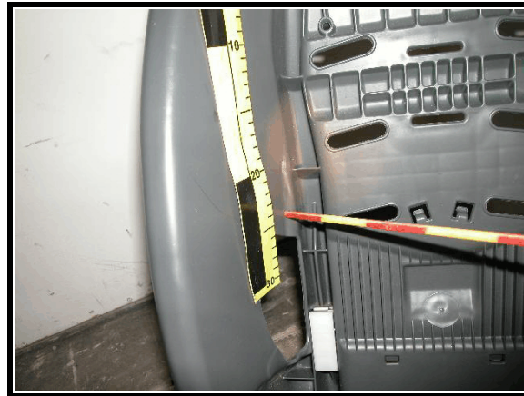
Figure 11. Close up of right seat back stress mark
