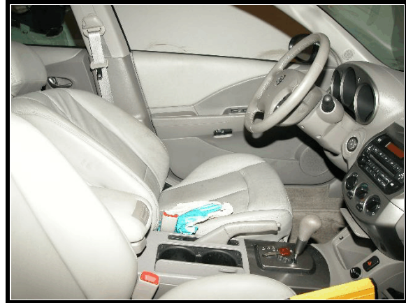
Figure 12. Driver's seat with deformed seat back
