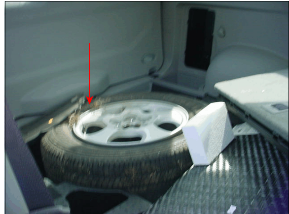
Figure 7: Insurance photo showing left front wheel in case vehicle's spare tire compartment, arrow shows grass jammed in bead
