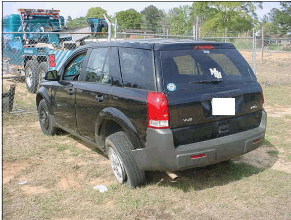
Figure 6: Insurance photo of case vehicle in tow lot showing condition of left rear wheel, spare tire mounted on left front
