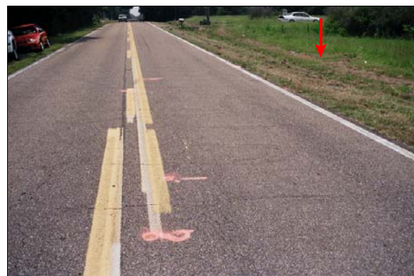
Figure 5: Case vehicle's left front yaw mark in foreground between paint dots, right rear yaw mark in background between paint marks, arrow shows area of case vehicle's final rest
