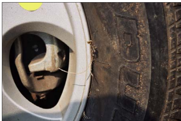
Figure 12: Grass jammed in bead of case vehicle's right front tire
