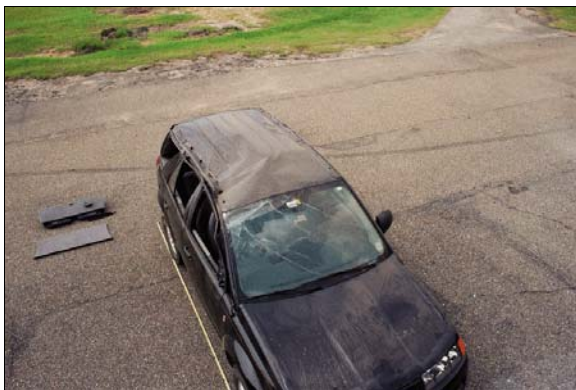
Figure 10: Top view of the crush to case vehicle's roof, roof side rails and right windshield header
