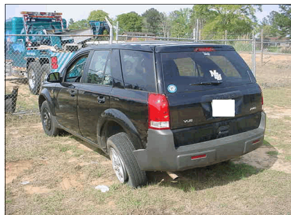
Figure 22: Insurance photo of case vehicle in tow lot showing condition of left rear wheel
