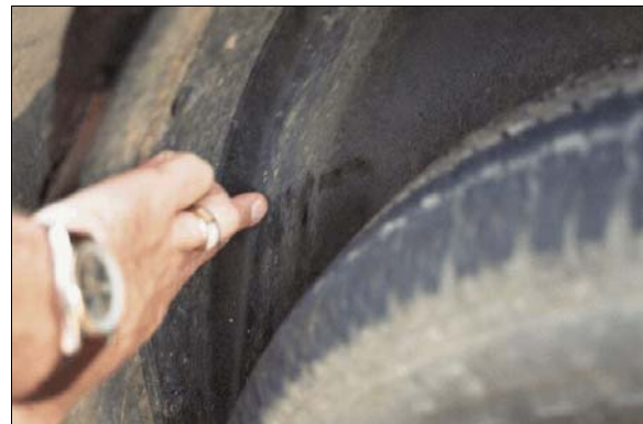
Figure 21: Scuff at front of left rear wheel house from contact by left rear tire
