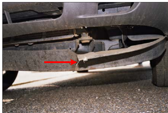
Figure 15: Damage to the left portion of case vehicle's front air scoop, blade of grass in mounting screw at center of photo
