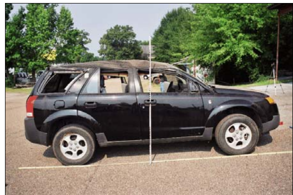
Figure 11: Overview of right roof side rail crush, vertical scale increments in tenths of foot
