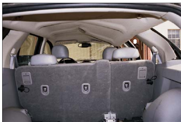
Figure 18: Intrusion of case vehicle’s roof, right roof side rail and right B and C pillars
