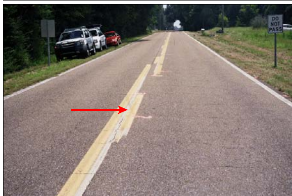
Figure 4: View southeast to case vehicle's yaw path, paint marks on center of roadway show yaw marks, arrow shows left rear yaw mark on centerline and no passing line
