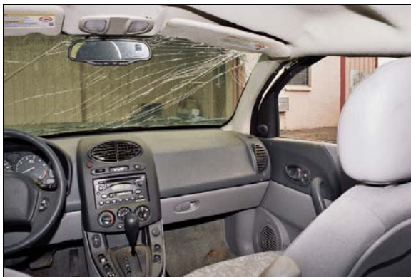
Figure 25: Overview of case vehicle's instrument panel, front right air bag located above glove box door
