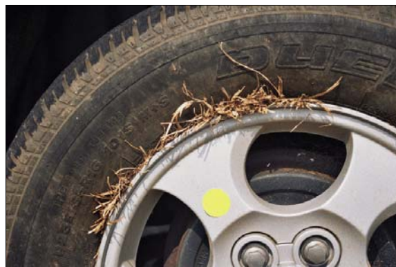
Figure 13: Grass jammed in bead of case vehicle's right rear tire
