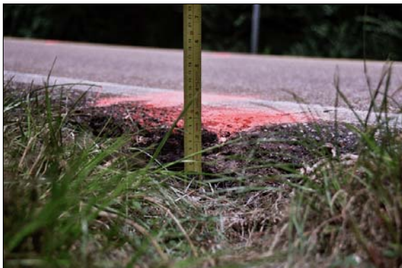
Figure 8: Remnants of divot from case vehicle's left front wheel, tape measure at bottom of divot
