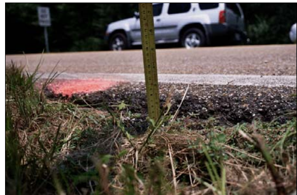
Figure 9: Remnants of divot from case vehicle's left rear wheel, tape measure at bottom of divot
