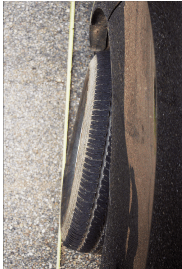
Figure 23: Top view of case vehicle's left rear wheel showing it angled to the right, outer treads abraded
