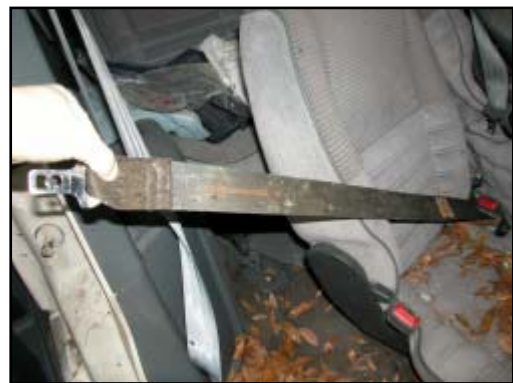
Figure 11. View of fully extended lap belt for the second row center position
