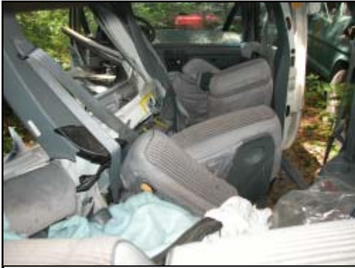
Figure 7. Longitudinal view from rear showing severe deformation and intrusion
