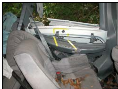
Figure 9. View of occupant contact on the left side panel
