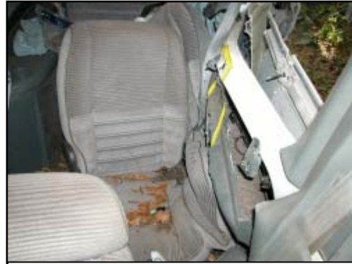
Figure 8. View of second row bench seat showing rotation and compression of the left seat
