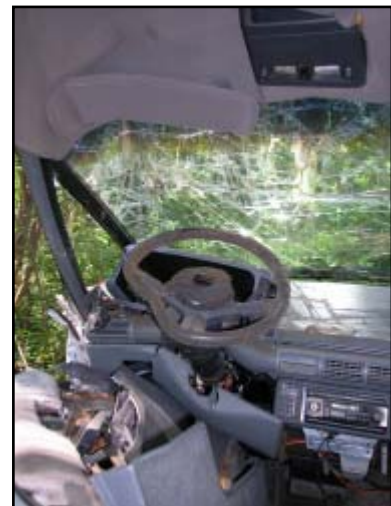
Figure 6. View of deformation and intrusion into the driver's position
