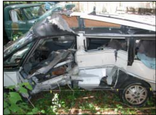
Figure 5. Overhead view of left side damage and roof separation
