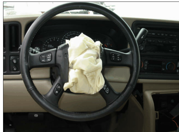
Figure 11: Case vehicle’s steering wheel and driver air bag module flaps
