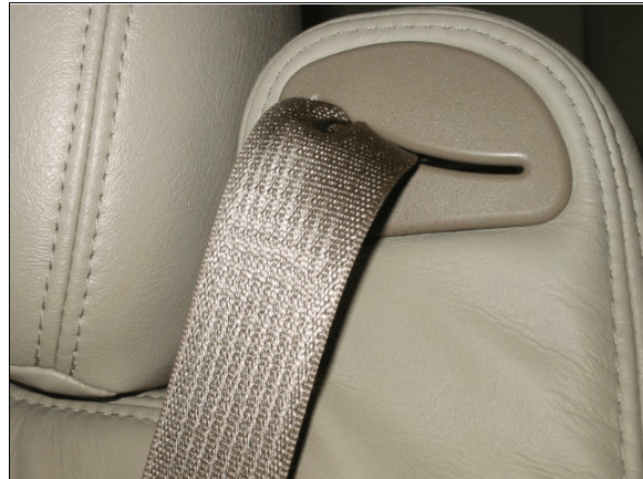
Figure 13: Case vehicle driver's shoulder belt jammed in the shoulder belt guide
