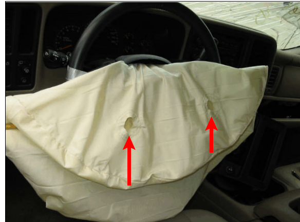
Figure 10: Location of case vehicle’s driver air bag vent ports (arrows)
