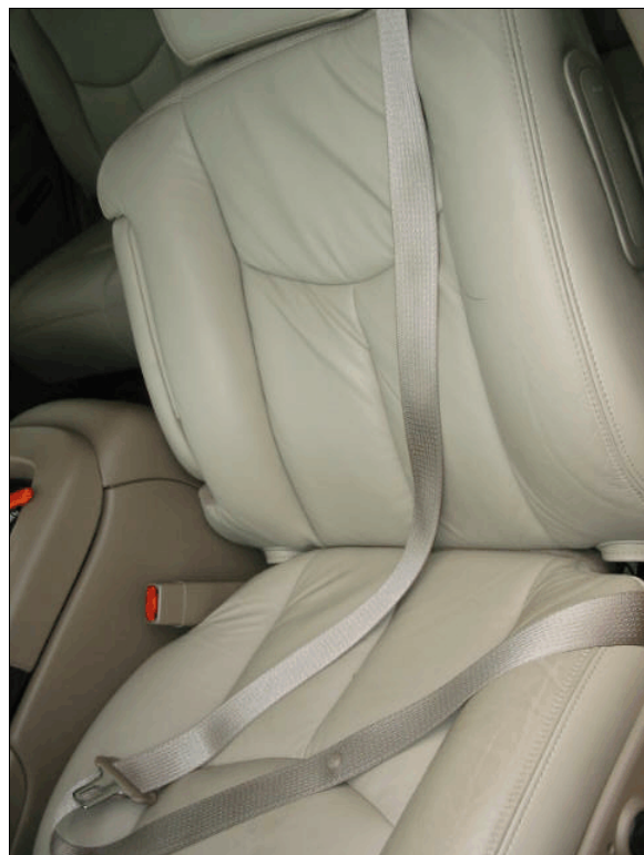
Figure 14: Overview of case vehicle driver's lap and shoulder belt in its jammed condition
