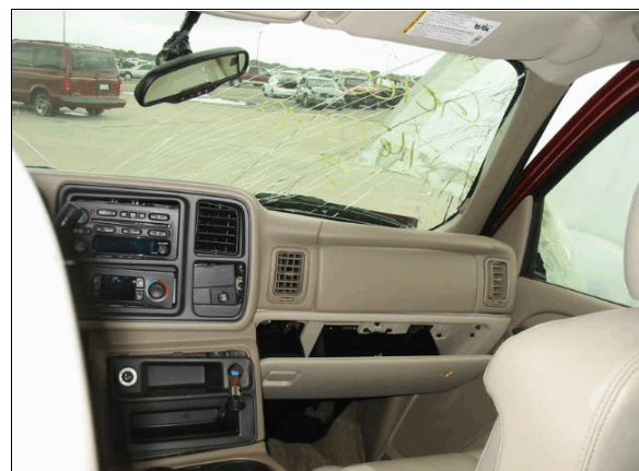
Figure 12: Case vehicle’s front right air bag module door located above glove box door
