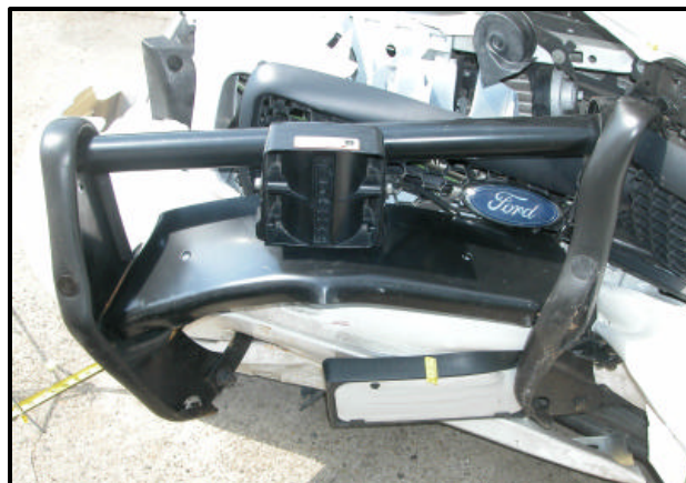
Figure 7: Close-up of the deformed push bumper.
