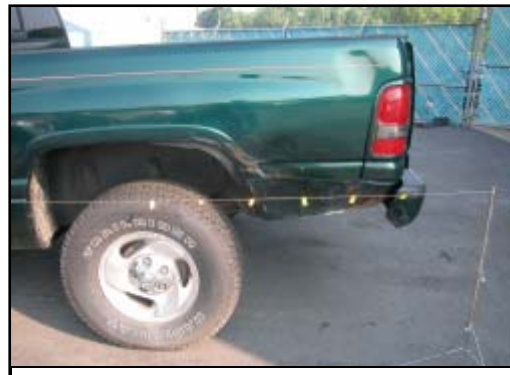
Figure 10. Left crush profile for secondary impact.
