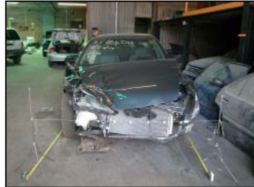
Figure 7. Upper radiator crush profile.
