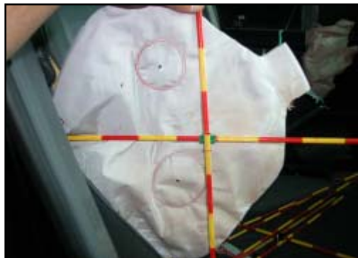
Figure 15. Deployed right seatback mounted side impact air bag.
