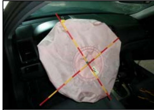
Figure 12. Deployed driver's frontal air bag.
