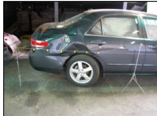
Figure 8. Crush profile for secondary impact.
