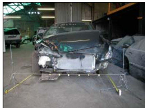
Figure 6. Lower radiator crush profile.
