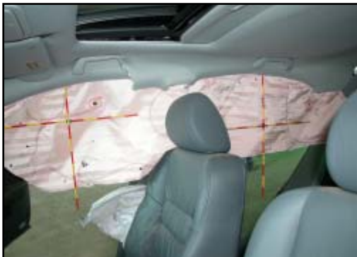
Figure 13. Overall view of deployed right side IC.
