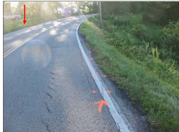
Figure 5: View west to second right rear yaw mark on north edge line of roadway and in grass, red arrow shows location of crash
