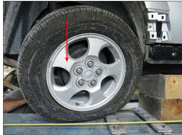
Figure 19: Right rear wheel, dirt on lug nuts and rim, arrow shows scratches on rim
