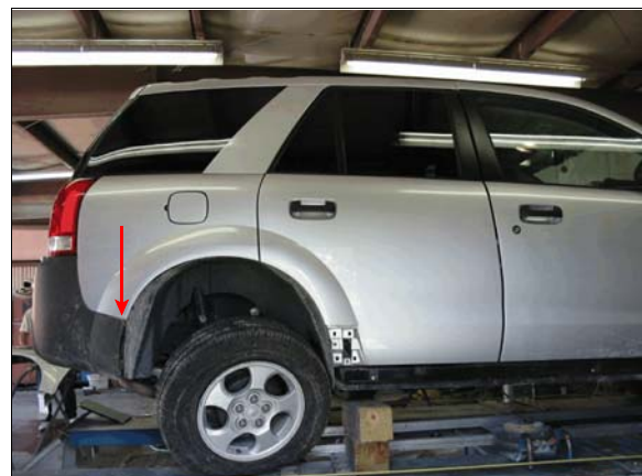
Figure 13: Overview of case vehicle's right side doors, right rear wheel and quarter panel, arrow shows grass/dirt jammed in quarter panel seam
