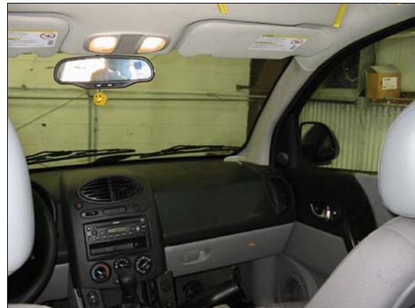
Figure 20: Front right air bag located in middle of instrument panel above glove box door
