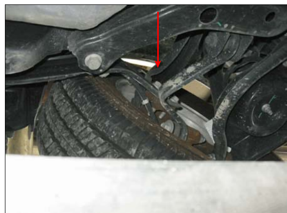
Figure 17: Damage to right rear suspension, toe link bent in V-shape, right rear tire against bent trailing arm, arrow shows upper control arm
