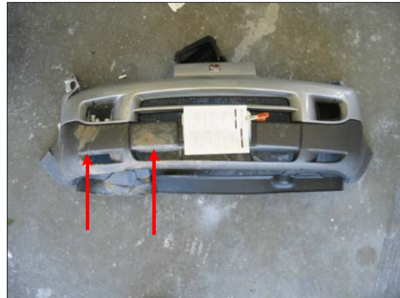
Figure 8: Case vehicle’s front bumper cover showing dirt transfer and ground contact damage to right half of the bumper cover
