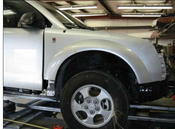
Figure 11: Direct damage scratches began at front of right front fender, grass in right front wheel bead
