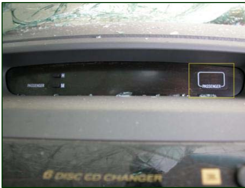
Figure 10. Passenger air bag indicator light for CAC safety system.
