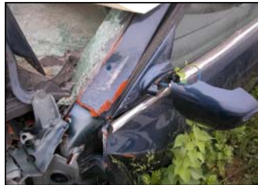
Figure 6. Damage from the mailbox impact.
