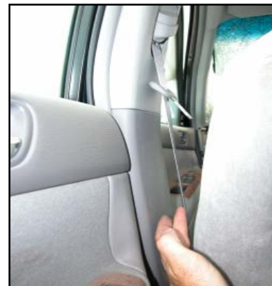
Figure 12. Stowed and taut position of the driver's safety belt webbing due to the fired
