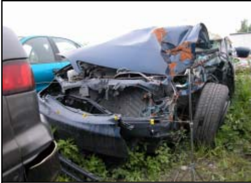
Figure 7. Front left corner damage from the utility pole impact.
