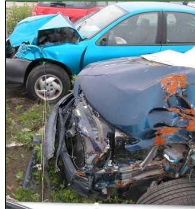
Figure 8. Lateral view depicting the extent of frontal crush.
