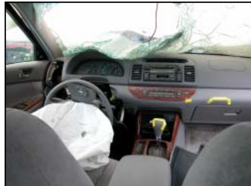
Figure 9. Overall view of the driver's trajectory and contact points.
