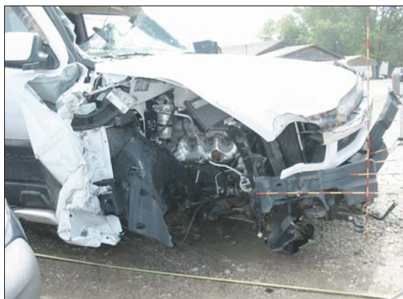
Figure 9: Damage to case vehicle from impact with Chevrolet Silverado’s towed training unit; crush measurements taken to bumper backing bar
