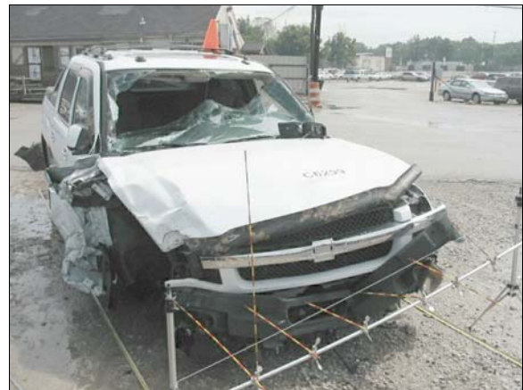
Figure 2: Damage to front right corner of case vehicle from impact to back of Silverado's towed trailing unit, each stripe on rods is 5 cm (2 in)
