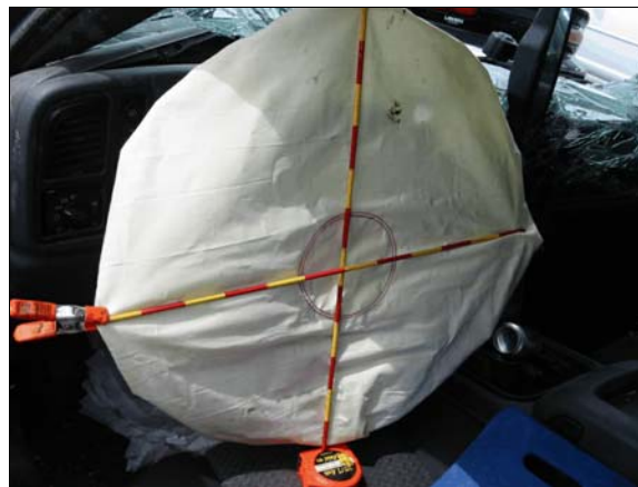
Figure 14: case vehicle's driver air bag, each stripe on rods is 5.0 centimeters (2.0 inches)
