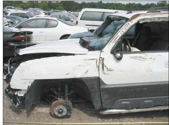
Figure 6: Rollover damage to case vehicle's left fender and left front door
