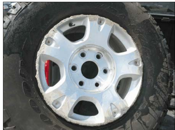
Figure 4: Pavement grinding on rim of case vehicle's left front wheel
