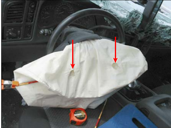
Figure 15: Case vehicle's driver air bag vent ports and steering wheel
