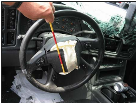
Figure 13: Case vehicle's driver air bag cover flaps
