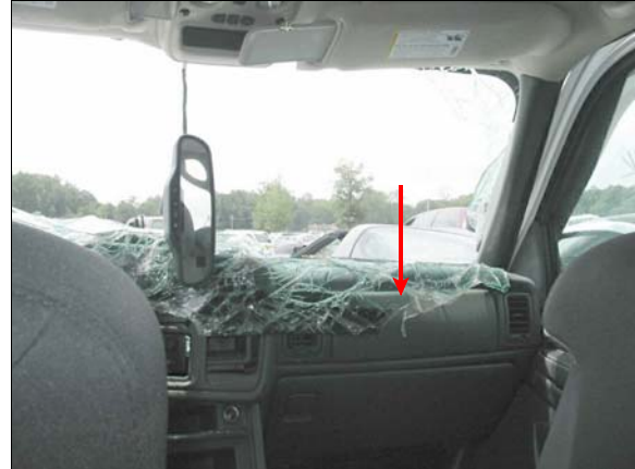
Figure 16: Case vehicle's front right air bag is located in the middle of the instrument panel above the glove box door.
