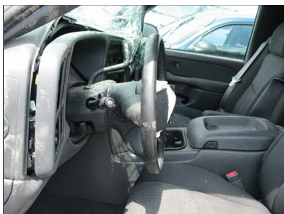
Figure 11: Case vehicle’s steering column and steering wheel showing lack of deformation
