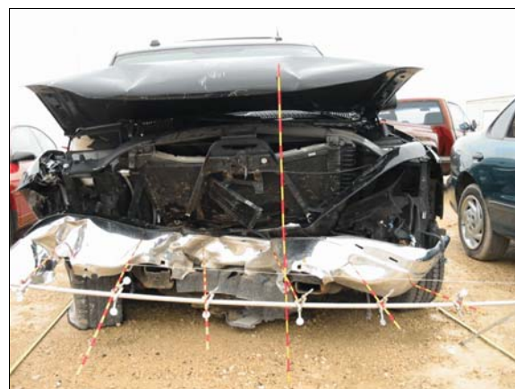
Figure 6: Direct damage to front of case vehicle from impact with Chevrolet
