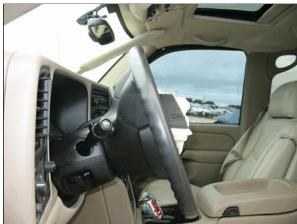
Figure 9: Case vehicle's steering wheel and steering column showing lack of deformation
