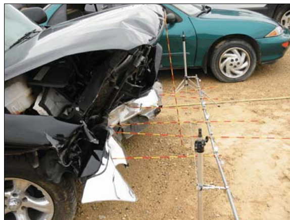
Figure 7: Crush to front of case vehicle, each stripe on rods is 5.0 centimeters (2.0 inches)
