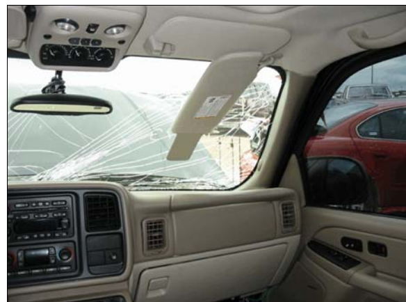
Figure 14: Overview of case vehicle's front right instrument panel, front right air bag located above glove box door
