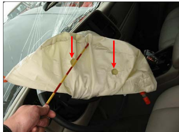
Figure 13: Case vehicle's driver air bag vent ports at top of air bag
