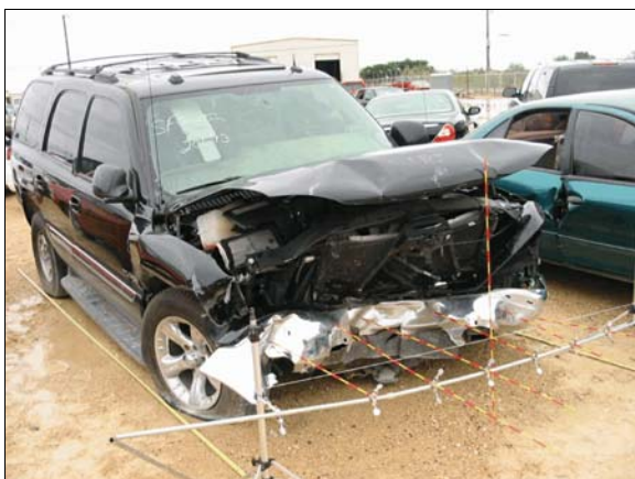
Figure 4: Overview of damage to front of case vehicle from impact with the Chevrolet, each stripe on rods is 5 cm (2 in)
