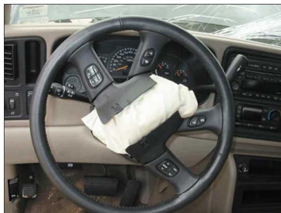
Figure 11: Case vehicle's steering wheel and air bag module cover flaps, steering wheel is rotated counterclockwise approximately 120 degrees
