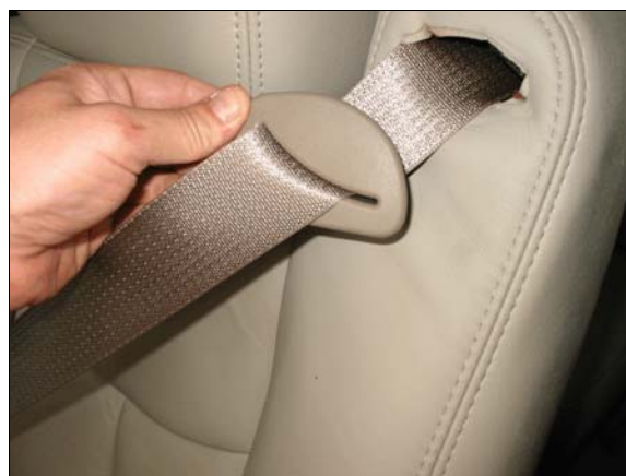
Figure 15: Case vehicle driver's shoulder belt guide pulled out of the seat
