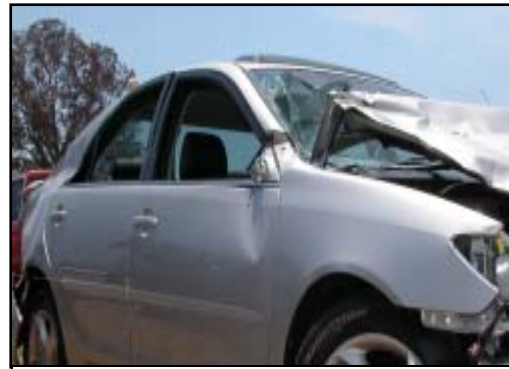
Figure 3. Right side damage from the impact with the lower edge of the
