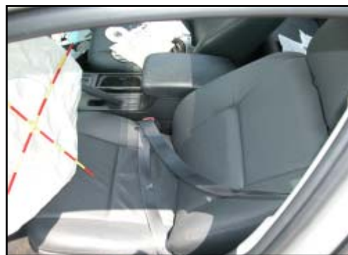
Figure 10. Driver's safety belt restricted in used position due to the fired pretensioner.
