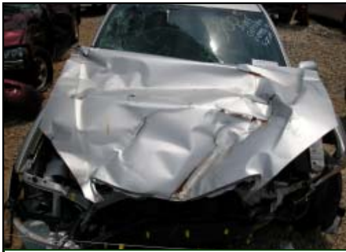
Figure 3. Damage to the top surface of the hood.
