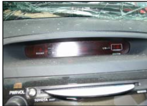
Figure 8. Front right air bag indicator light and safety belt minder light.
