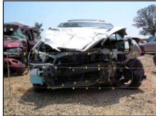
Figure 6. Frontal damage from the extended height Jersey barrier. View of the three crush profiles documented for this impact.
