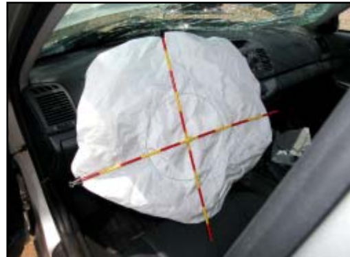
Figure 9. Deployed driver's frontal air bag.
