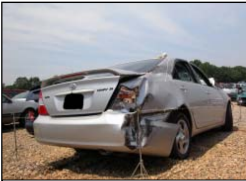
Figure 5. Rear damage from the impact with the trailer wheels.
