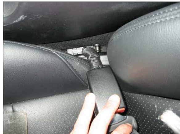
Figure 14: Compression of driver's seat belt buckle stalk due to activation of the seat belt pretensioner (case photo # 31)
