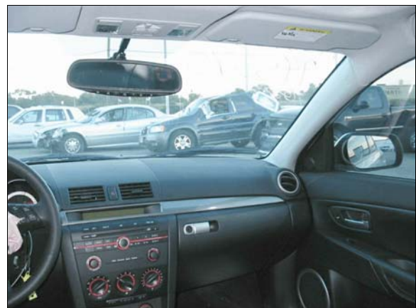
Figure 12: Front right air bag located in top of instrument panel above glove box door (case photo #35)
