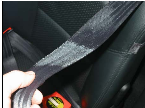
Figure 13: Load mark on driver's shoulder belt (case photo #30)
