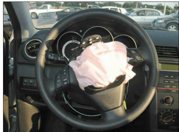
Figure 11: Overview of air bag module flaps (case photo # 22)
