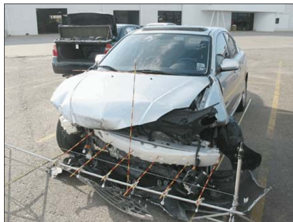
Figure 6: Overview of damage to front of case vehicle from impact with the concrete median barrier (case photo #10)
