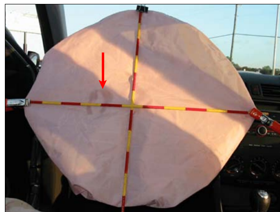
Figure 8: Case vehicle’s driver air bag, arrow shows stain in the air bag material (case photo #25)
