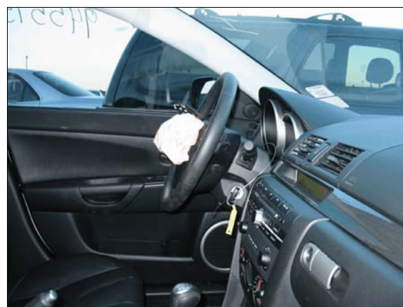
Figure 9: Overview of steering wheel and steering column showing lack of deformation (case photo #38)
