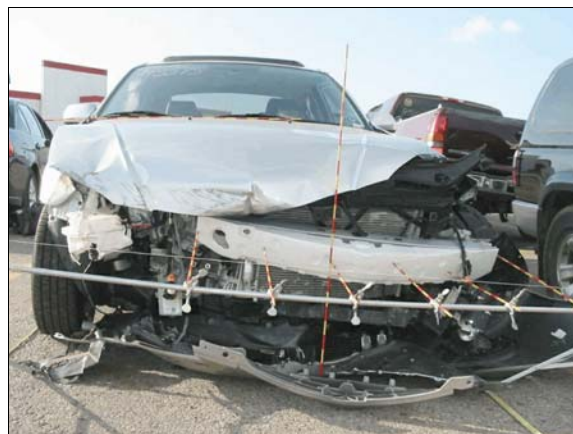
Figure 4: Damage to front of case vehicle [each stripe on rods is 5 cm (2 in)] from impact with the median barrier (case photo #08)
