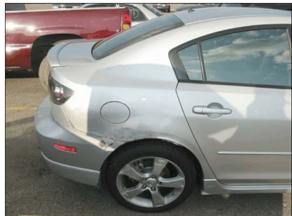
Figure 2: Damage to right quarter panel and right rear wheel due to sideswiping the concrete longitudinal barrier (case photo #15)
