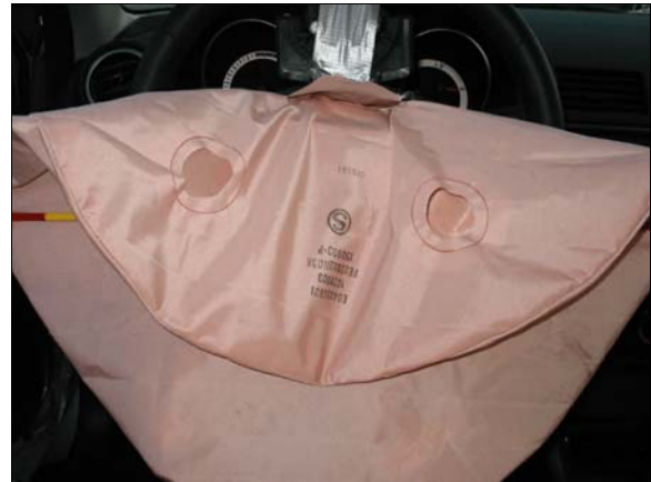
Figure 10: Case vehicle's driver air bag vent ports (case photo # 27)
