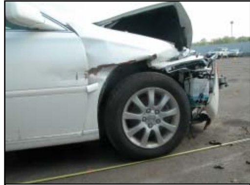
Figure 5. Right front fender damage from guardrail
