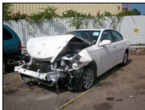
Figure 4. Frontal damage to the 2004 Lexus ES 330
