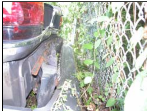
Figure 8. Lateral view from left along damaged rear bumper beam
