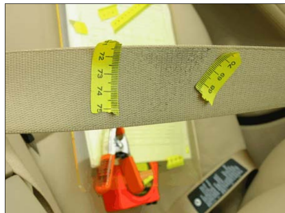
Figure 17: Plastic transfer from D-ring on front right shoulder belt (case photo #42)
