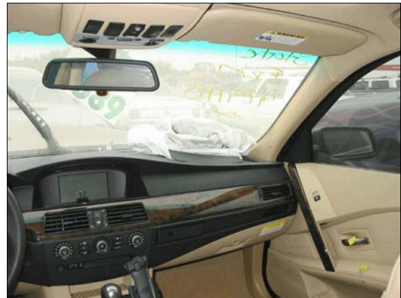
Figure 12: Overview of location of front right passenger air bag in top of right instrument panel (case photo #48)
