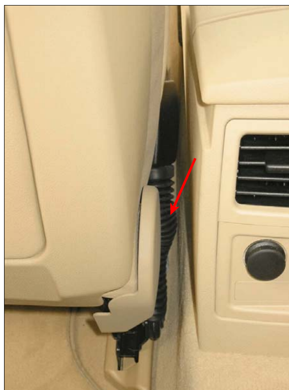
Figure 15: Arrow shows compression of driver's seat belt buckle stalk cover
