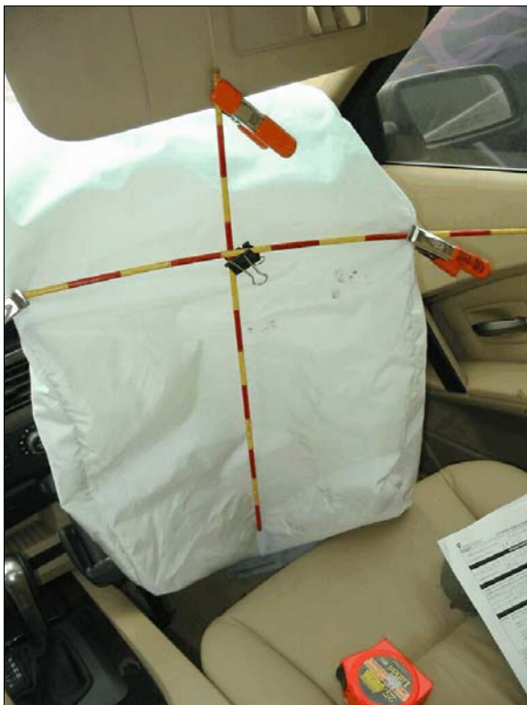
Figure 13: Front right passenger air bag, blood smears in right lower quadrant (case photo #32)
