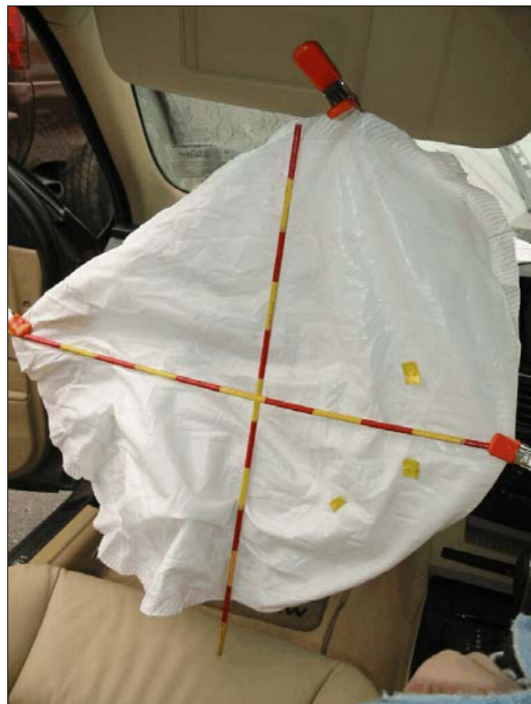
Figure 9: Driver's air bag, yellow tape shows area of probable makeup smears (case photo #28)
