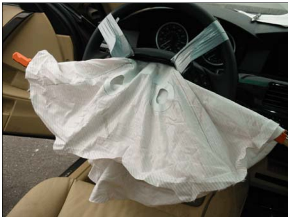
Figure 10: Driver's air bag vent ports (case photo #39)
