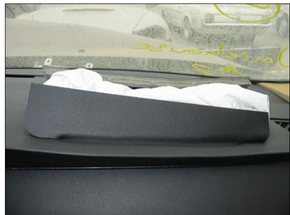
Figure 14: Front right air bag module cover flaps (case photo #37)
