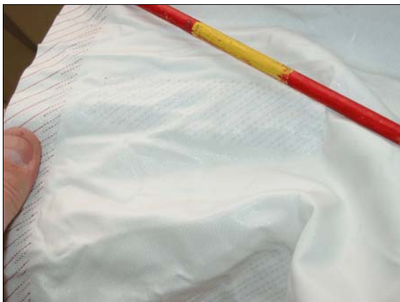
Figure 8: Close view of the bonding strips on the driver's air bag (case photo #31b)
