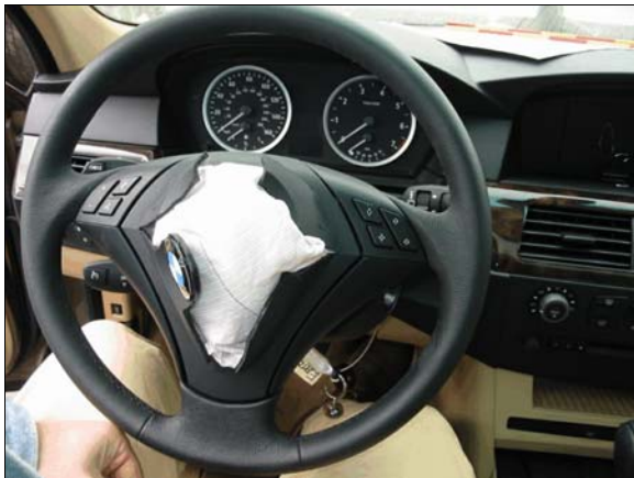
Figure 11: Driver's air bag module cover flaps (case photo #26)
