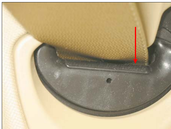
Figure 16: Abrasions (arrow) from the shoulder belt on the front right D-ring (case photo #45)
