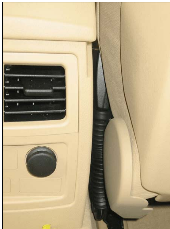
Figure 18: Compression of front right seat belt buckle stalk cover (case photo #48a)
