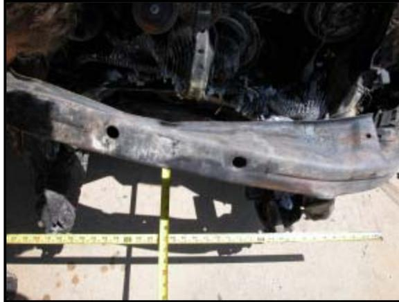
**Figure 14: Deformed lower frame caused by the scales in the CVPI trunk.**
