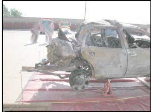
**Figure 8: Right view of the CVPI rear damage.**
