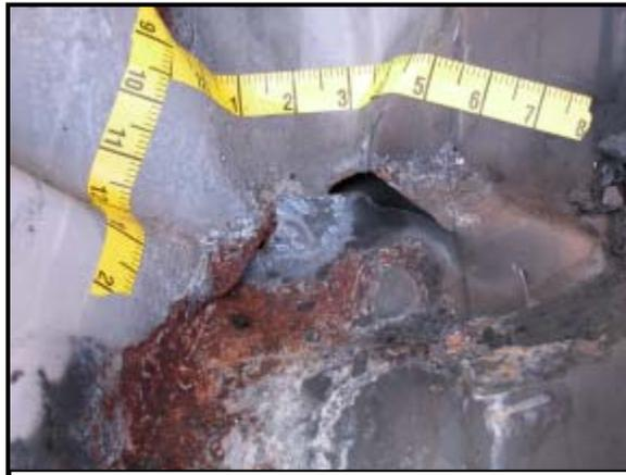
**Figure 20: Close-up view of the tank perforation.**
