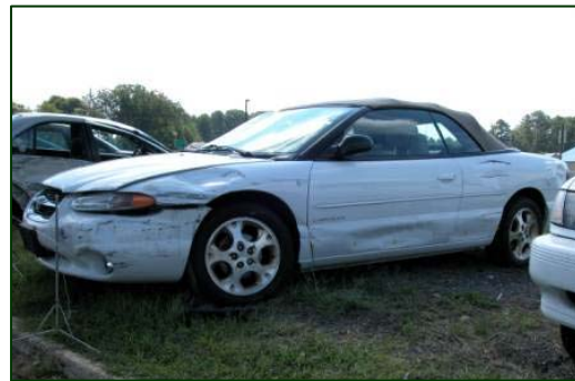
Figure 6. Right side damage from the secondary engagement.
