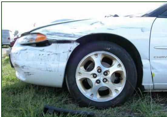
Figure 4. Initial impact damage to the left front fender area.
