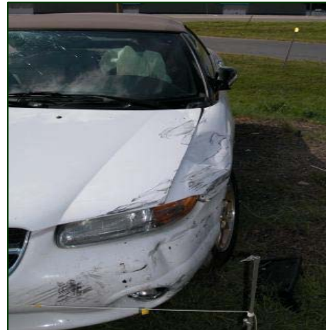
Figure 5. Longitudinal view documenting the lateral extent of crush.
