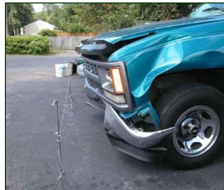
Figure 8. Lateral view documenting the extent of frontal crush.
