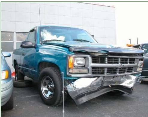
Figure 7. Front right view of the frontal damage to the 1998 Chevrolet pickup truck.
