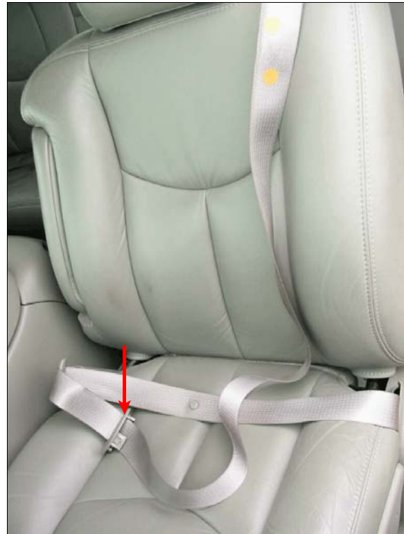
Figure 10: Overview of driver's seat and safety belt, orange dots show location of load mark on driver's shoulder belt, arrow shows displaced shoulder belt guide
