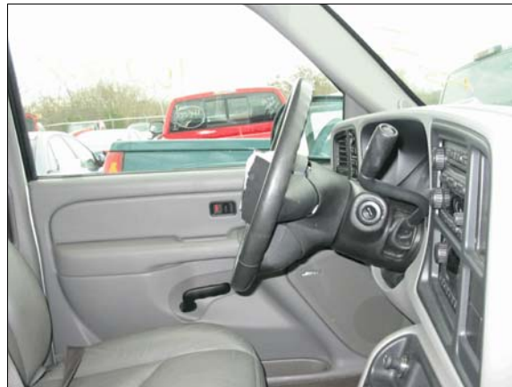
Figure 6: Steering wheel and steering column were not deformed
