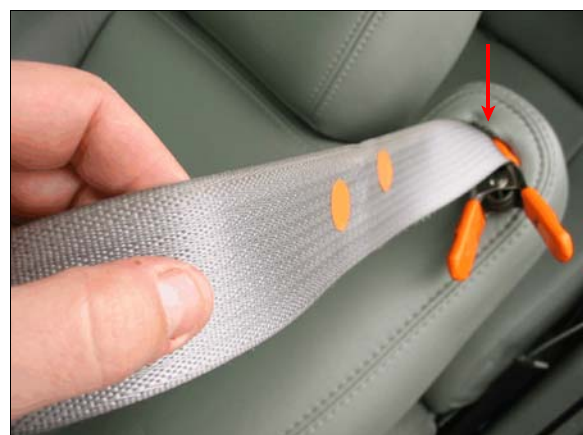
Figure 11: Close view of load mark on driver's shoulder belt, arrow shows installed location of displaced shoulder belt guide
