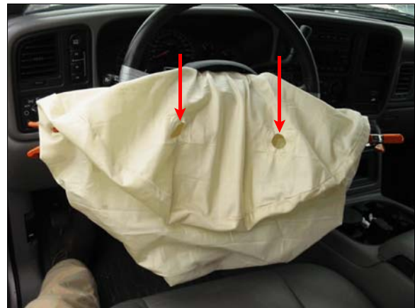
Figure 8: Back of driver's air bag, arrows show air bag vent ports
