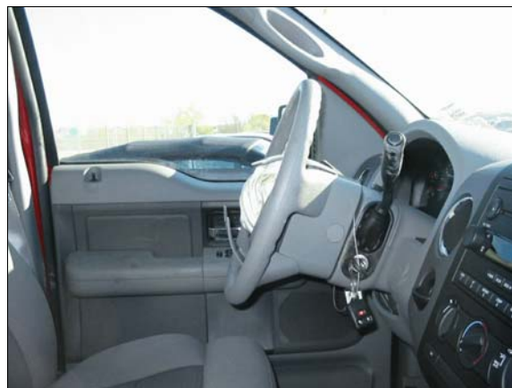
Figure 12: Case vehicle's steering column and steering wheel showing lack of damage
