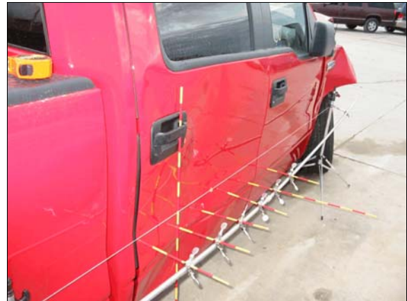
Figure 5: Side-slap damage to case vehicle's right rear door.
