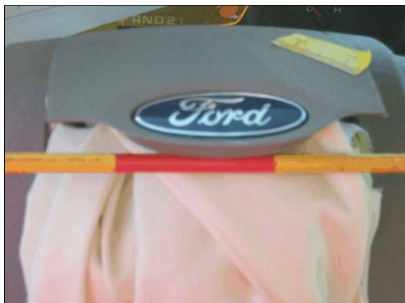
Figure 11: Tape shows scuff on upper air bag module cover flap
