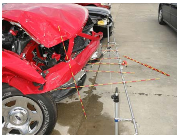
Figure 8: Crush to case vehicle's front bumper due to impact with the Oldsmobile, each stripe on rods in 5 cm (2 in)
