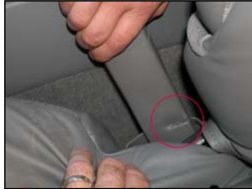
Figure 18. Laceration to safety belt sleeve from loading against seatback
