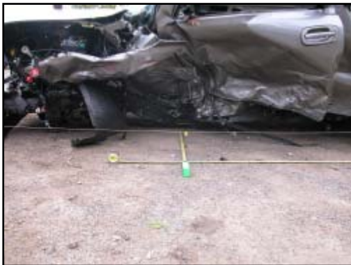
Figure 8. Forward aspect of the left frame rail crush.
