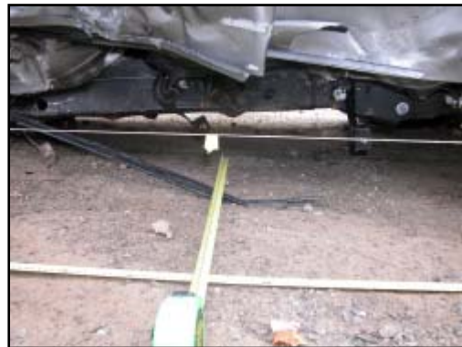
Figure 9. Rear aspect of the left frame rail crush.
