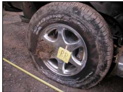
Figure 11. Right rear tire damage.
