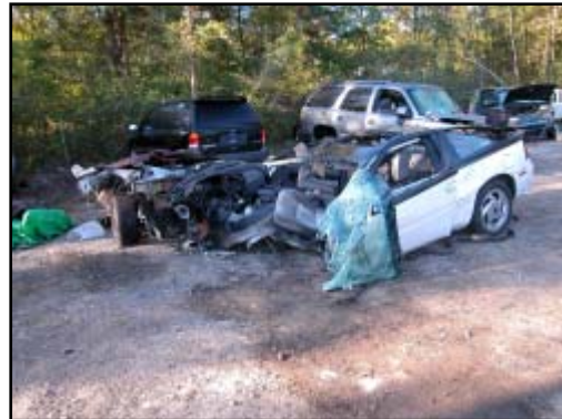
Figure 15. Left side structure torn from at impact.
