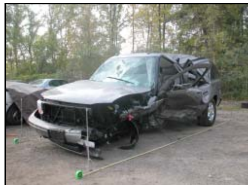
Figure 7. Damage from the impact with the Eagle.
