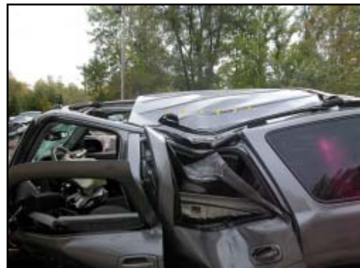
Figure 13. Left roof and roof side rail damage.
