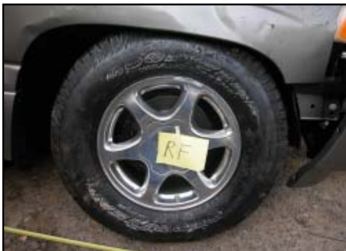
Figure 10. Right front tire damage. Note damage consisted of abrasions to the sidewall.
