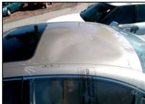
Figure 7. Overhead view of left rear roof damage
