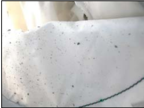
Figure 10. View of grey deposits on interior of air bag fabric
