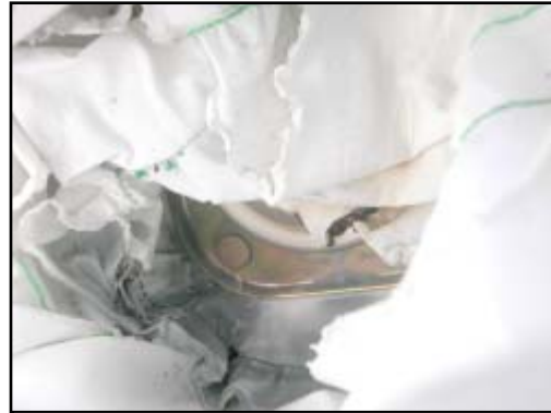
Figure 11. Bottom aspect of the inflator and grey deposits
