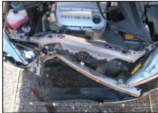
Figure 6. Overhead view of frontal crush
