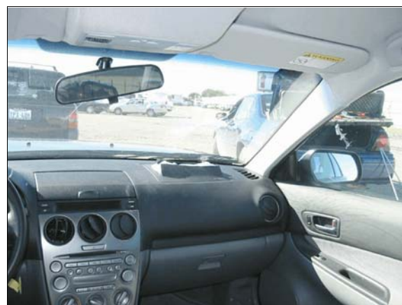
Figure 9: Overview of front right instrument panel, front right air bag in top of instrument panel
