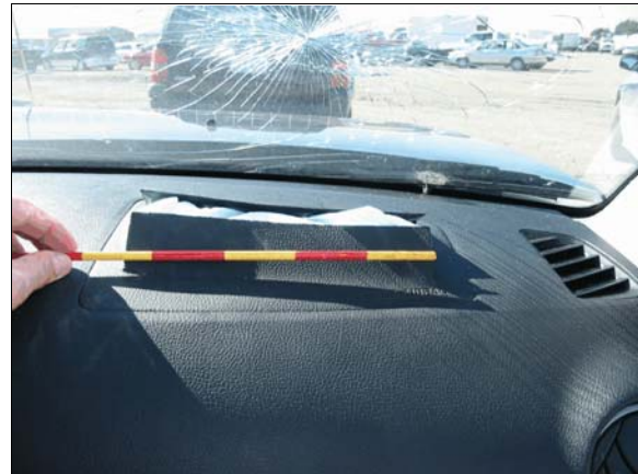
Figure 14: Front right passenger air bag module flaps and cracked windshield from air bag deployment
