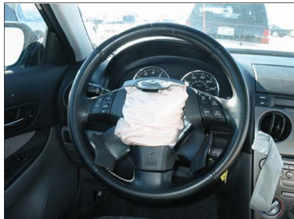
Figure 11: Case vehicle's steering wheel and air bag module flaps
