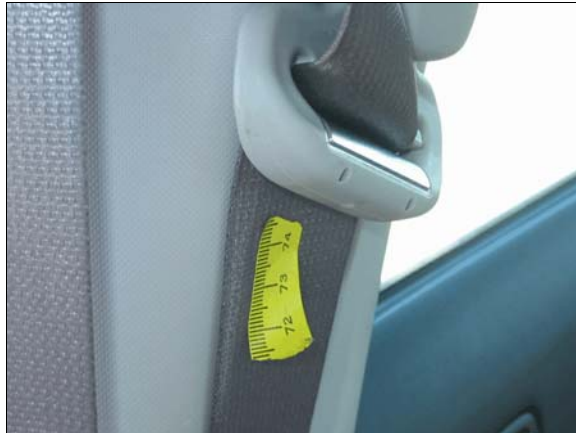
Figure 16: Load abrasion on front right passenger's shoulder belt, indicated by yellow tape
