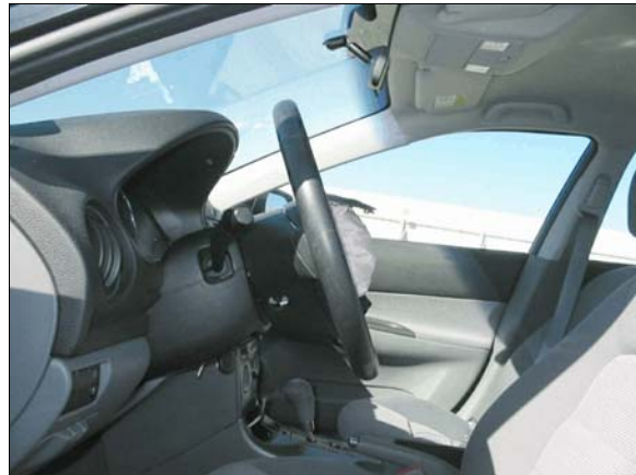
Figure 10: Case vehicle's steering column and steering wheel showing lack deformation
