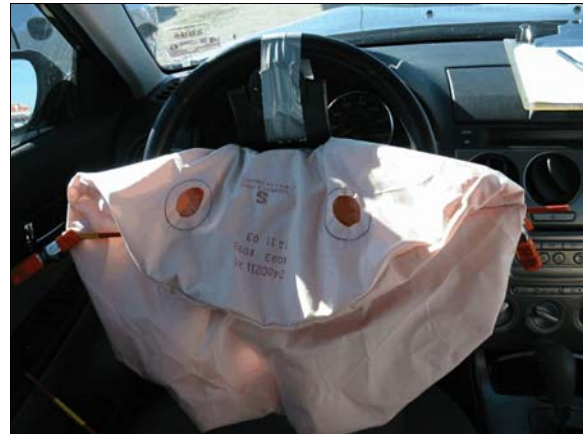
Figure 13: Top back portion of case vehicle's driver air bag showing vent ports
