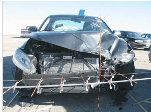
Figure 3: Damage to front of case vehicle due to impact with Ford and Toyota
