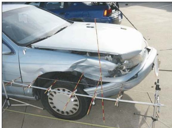
Figure 4: Damage to right fender of Ford Taurus due to impact with case vehicle, each stripe on rods is 5 cm (2 in)
