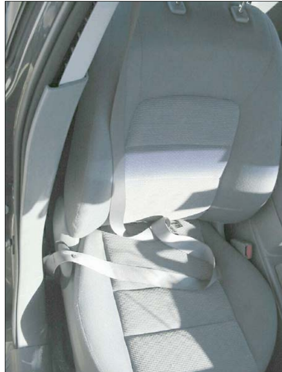
Figure 17: Front right passenger's safety belt, it would not spool out or retract
