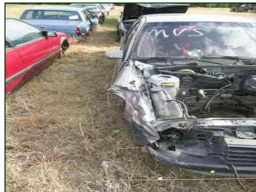
Figure 6. Front and right side damage to the Corsica.
