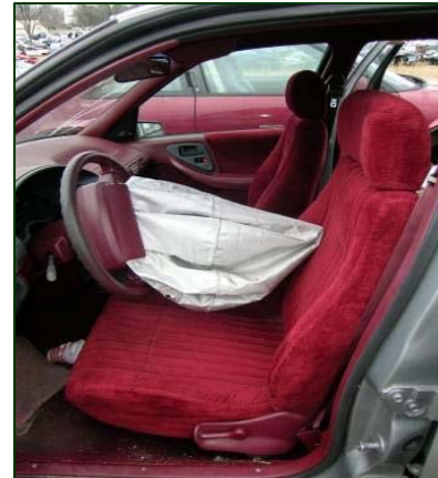
Figure 9. Rearward excursion of the driver's air bag into mid track seat position.
