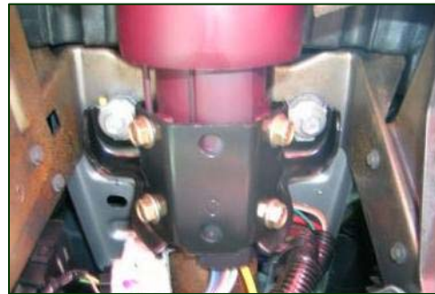
Figure 7. Steering column shear brackets; no separation
