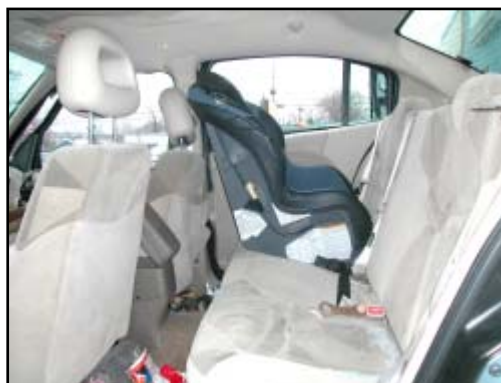
Figure 16. Post-crash position of the CSS during vehicle inspection
