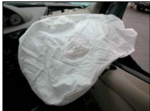
Figure 14. Deployed front right passenger's air bag
