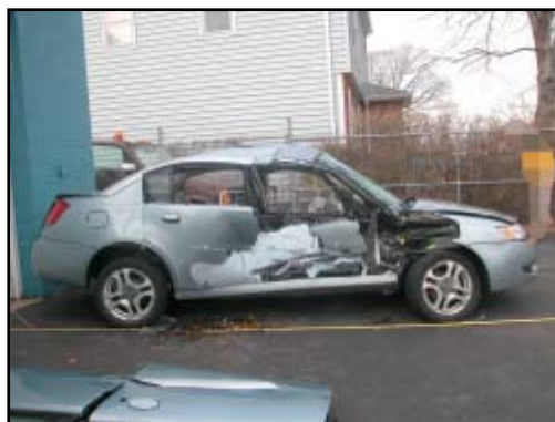
Figure 6. Lateral view of right side crush profile
