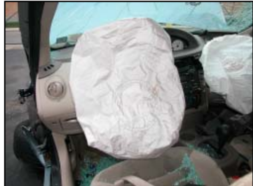
Figure 13. Deployed driver's air bag
