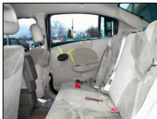
Figure 9. View of damaged right rear door and intrusion
