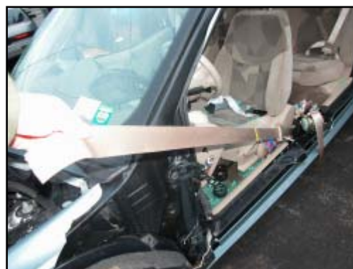
Figure 10. View of cut driver's safety belt
