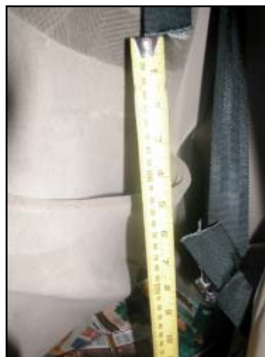
Figure 17. Post-crash gap between tether cuts
