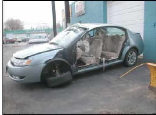
Figure 7. Left side view showing damaged left front wheel
