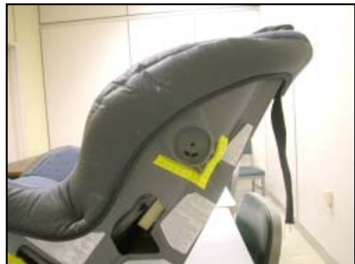
Figure 18. Left side damage to CSS
