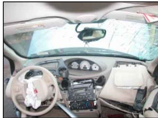
Figure 8. View of damaged instrument panel
