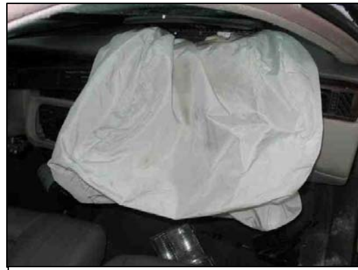
Figure 9 - Deployed front right passenger's air bag.
