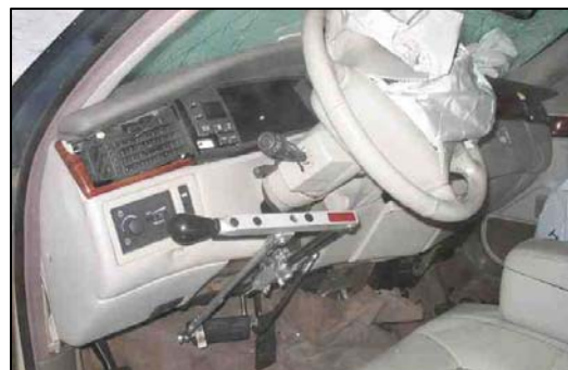
Figure 10 - Adaptive hand controls and indented instrument panel.
