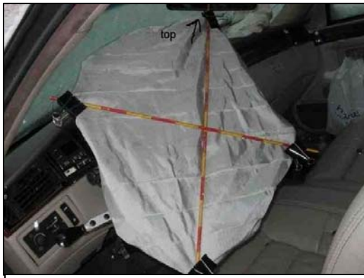
Figure 8 - Deployed driver's air bag.
