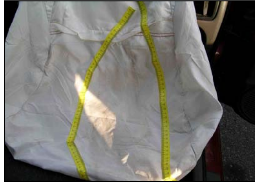
Figure 12 - Overall view of transfer evidence on the front right air bag.
