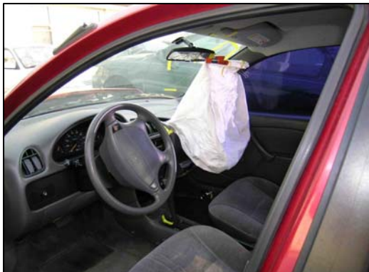
Figure 9 - Asymmetrical air bag deployment.
