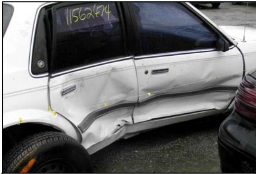
Figure 7 - Right side damage to the 1996 Buick Century.
