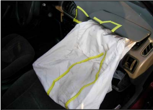
Figure 11 - Overall view of the transfer evidence on the front right air bag.
