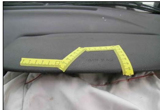
Figure 10 - Transfer evidence on the leading edge of cover flap.
