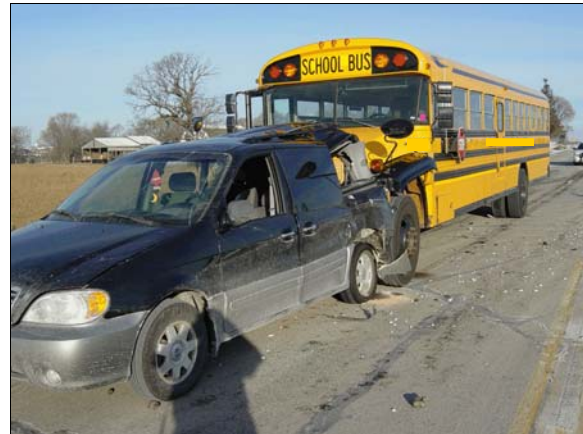
Figure 4: Final rest position of case vehicle and school bus and view of school bus' left front and left rear skid marks
