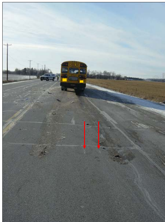
Figure 2: Police on-scene photo showing point of impact (arrows show gouges from case vehicle) and final rest position of school bus
