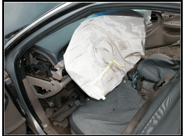
Figure 12. Deployed driver's air bag
