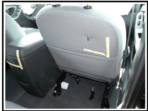
Figure 7. Contacts to right seat back and center console
