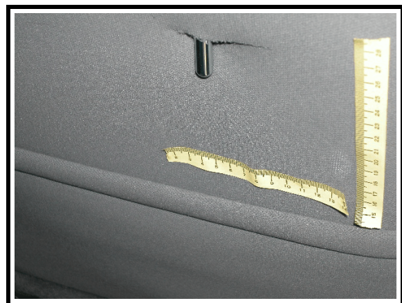
Figure 8. Closeup of contact and damage to right seat back
