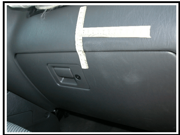
Figure 11. Closeup of contact to the right instrument panel and glove box
