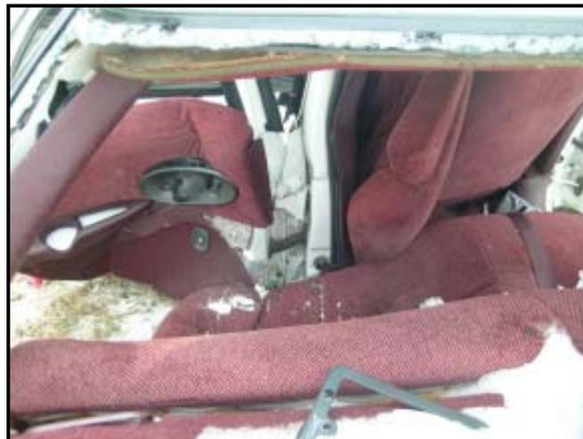
**Figure 12: Overhead view through the backlight of the rear seat intrusion.**
