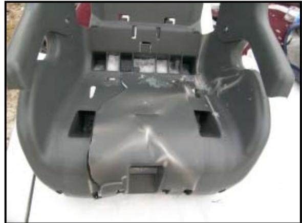
**Figure 16: Close-up view of the fractured base.**
