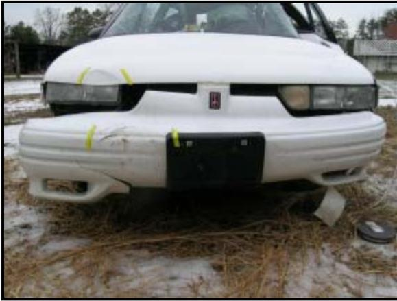
Figure 6: View of the fascia damage.
