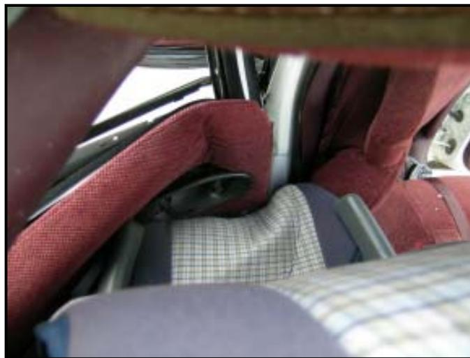
**Figure 17: Overhead view of the relationship between CSS in the rear left position and the left side intrusion.**
