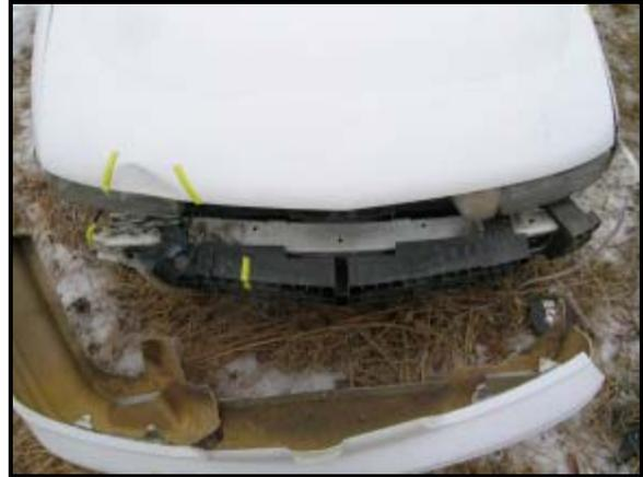
Figure 7: View of the reinforcement bar.
