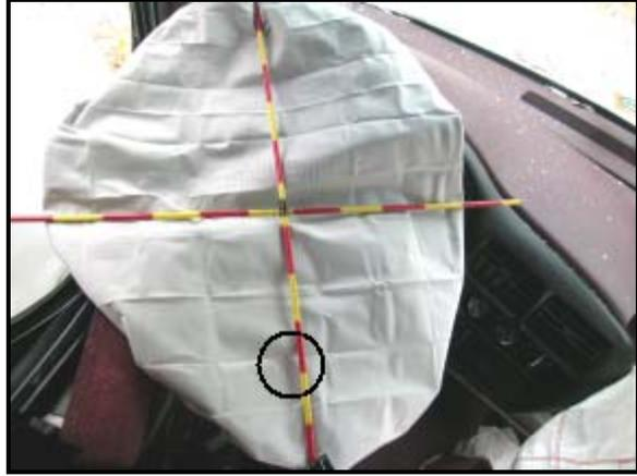
**Figure 13: Deployed driver air bag.**
