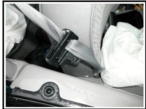
Figure 7. Front right passenger seat belt, webbing trapped in latch plate
