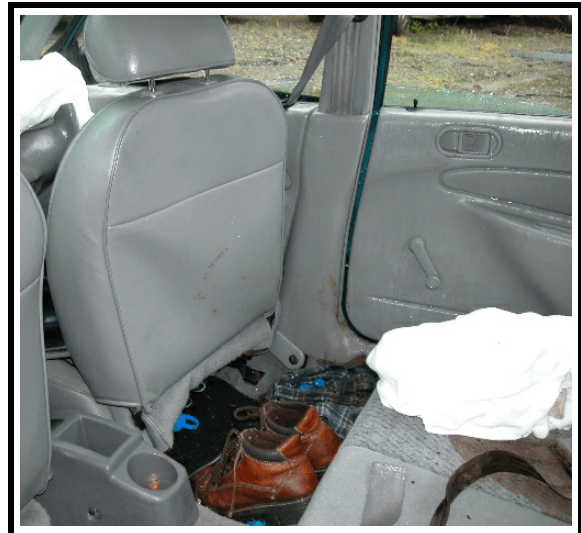
Figure 15. Second row right seat position, deformation to front right seat back
