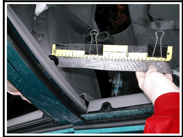
Figure 6. Loading to driver's seat belt—viewed through left rear window
