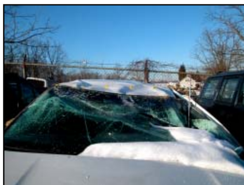
Figure 6. Windshield header showing vertical deformation
