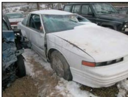
Figure 5. Right side damage to the Cutlass Supreme
