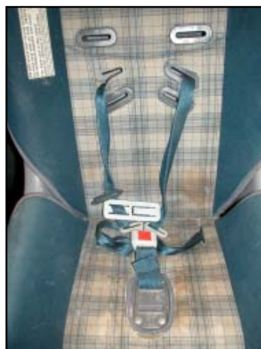
Figure 13. View of harness system
