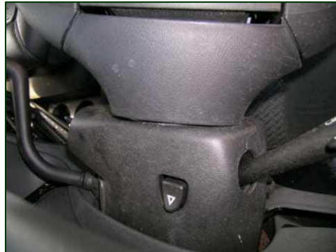
Figure 8. Bending of steering wheel flange.
