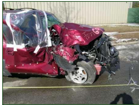
Figure 5. Lateral view of the extent of crush to the right A-pillar.
