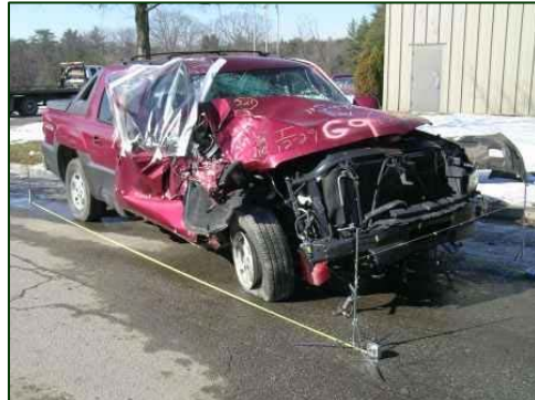
Figure 1. Front right corner damage to the 2004 Chevrolet Avalanche.
