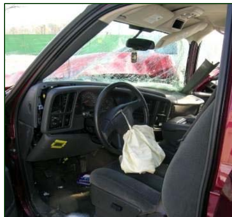
Figure 9. Deployed Stage 1 driver's air bag.
