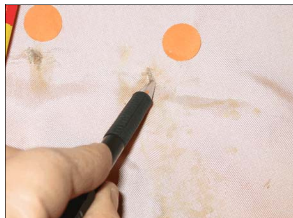
Figure 14: Close view of small holes in driver's air bag
