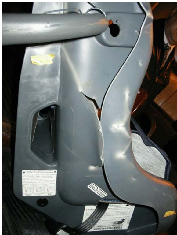
Figure 21: Stress marks and damage to right side of 2 nd seat center child seat
