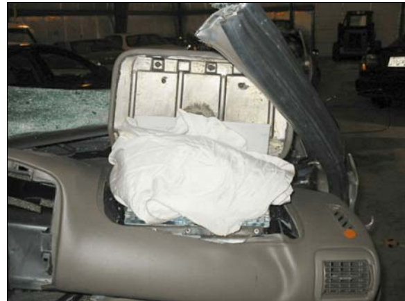
Figure 15: Location of front right air bag in top of instrument panel
