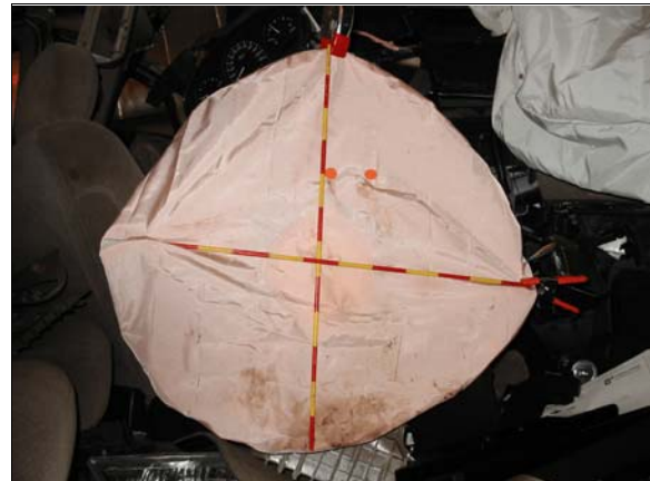
Figure 12: Case vehicle's driver air bag, orange dots show small holes in air bag
