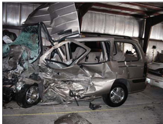
Figure 8: Damage to case vehicle's left side doors from impact with the Pontiac
