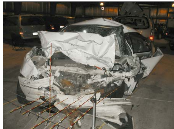
Figure 4: Damage to Pontiac from impact with case vehicle, each increment on rods is 5 cm (2 in)
