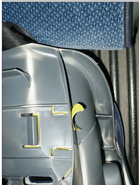
Figure 18: Stress marks and cracks to back, upper right portion of 2nd seat center child seat
