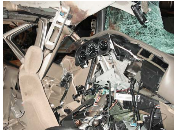
Figure 10: Intrusion into driver's occupant space
