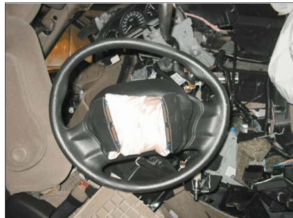
Figure 11: Deformation to case vehicle's steering wheel and overview of air bag module flaps
