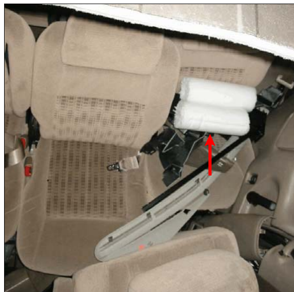
Figure 22: Intrusion of the case vehicle driver's seat into the 2 nd seat center and left seat positions; arrow shows pool noodles used to position child seats
