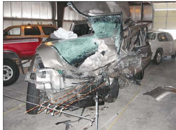
Figure 5: Damage to case vehicle from impact with the Pontiac
