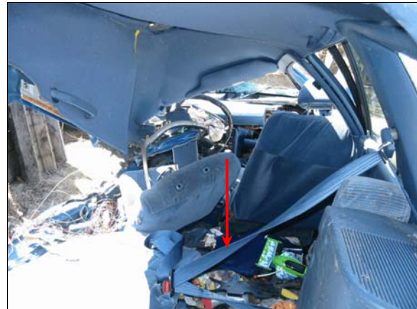
Figure 9: Overview of case vehicle's roof intrusion, back right safety belt found buckled (arrow) and was observed to be buckled in police on-scene photos
