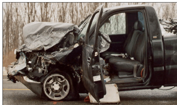
Figure 21: Police on-scene photo of front damage to Chevrolet
