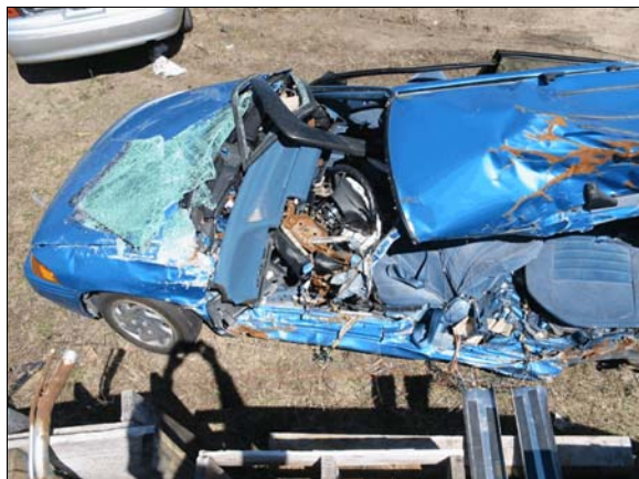
Figure 5: Damage to left side of case vehicle due to impact with the Chevrolet
