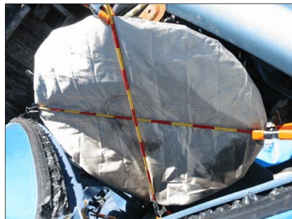
Figure 10: Case vehicle's driver air bag, each increment on rods in 5 cm (2 in)
