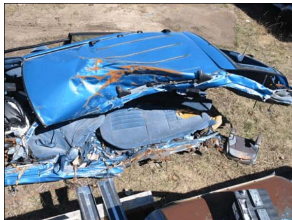
Figure 6: Damage to left side of case vehicle due to impact with the Chevrolet
