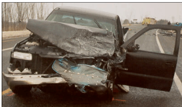
Figure 20: Front damage to Chevrolet from impact with left side of case vehicle, case vehicle's left front door sheet metal stuck to front bumper
