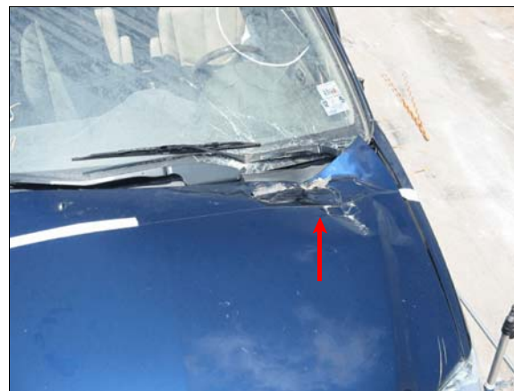
Figure 22: Damage to Lexus' hood and windshield due to fire hydrant impact during the rollover
