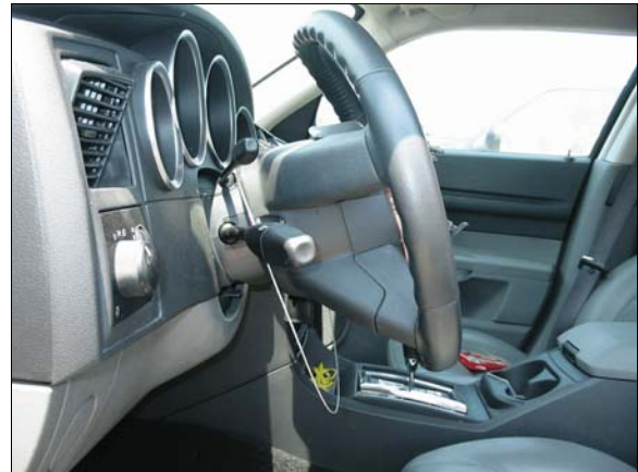
Figure 13: Left side view of deformation to steering wheel rim
