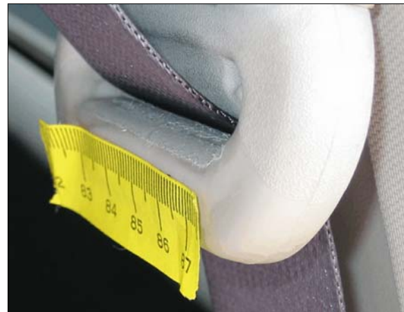
Figure 18: Load marks in case vehicle driver’s safety belt D-ring
