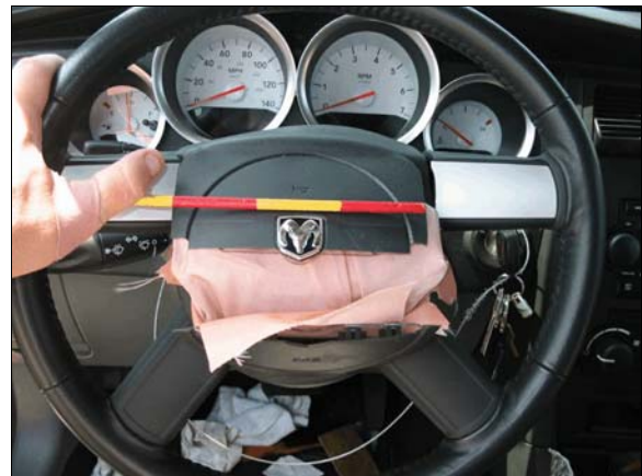
Figure 14: Case vehicle's driver air bag module cover flaps
