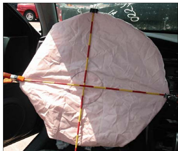
Figure 15: Case vehicle's deployed driver's air bag
