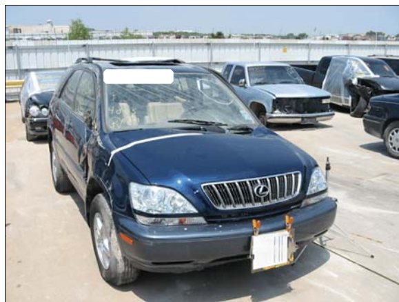
Figure 21: Overview of damage to the roof and right side of the case vehicle due to the rollover
