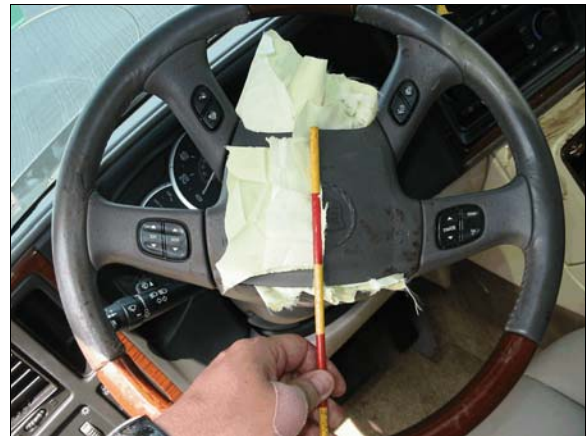
Figure 14: Driver's air bag was cut out of case vehicle, steering wheel upside down, measurement rod shows height of cover flaps, each increment on rod is 5 cm (2 in)
