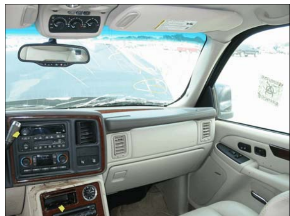
Figure 15: Front right air bag located in middle of right instrument panel above glove box door
