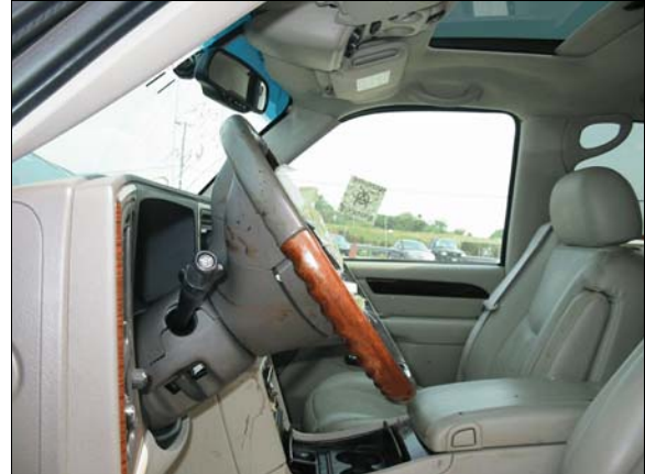
Figure 13: Left side view of case vehicle's steering column and steering wheel showing lack of deformation, steering column moved to full up position
