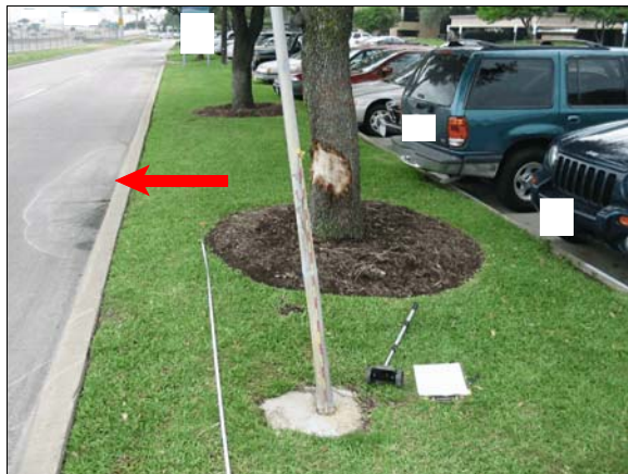
Figure 4: Impacted sign post and tree, arrow shows fluid spill stain on roadway at case vehicle’s final rest location, each increment on rod is 5 cm (2 in)
