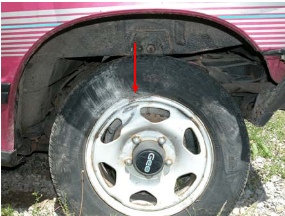
Figure 5: Damage to left rear wheel (arrow) from impact with header wall
