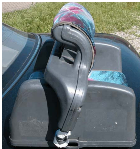
Figure 25: Left side view of child seat showing swivel mount for shield
