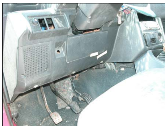
Figure 17: Tapes show location of probable knee scuffs on lower instrument panel
