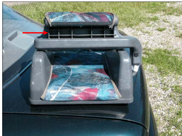
Figure 23: Front of child seat, arrow shows guide for safety belt
