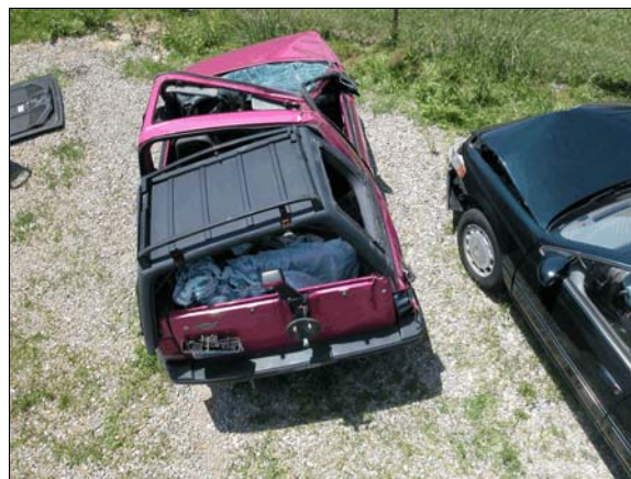
Figure 16: Top view of damage to case vehicle
