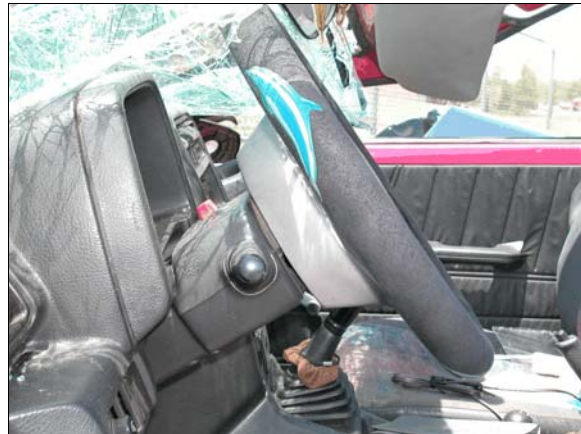
Figure 22: Left side view of steering column and steering wheel showing lack of deformation
