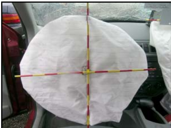
Figure 8: Deployed driver air bag.
