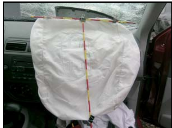
Figure 9: Deployed front passenger air bag.
