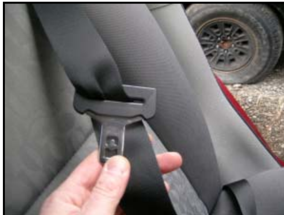
Figure 7: Left rear restraint webbing gathered in the latch plate.
