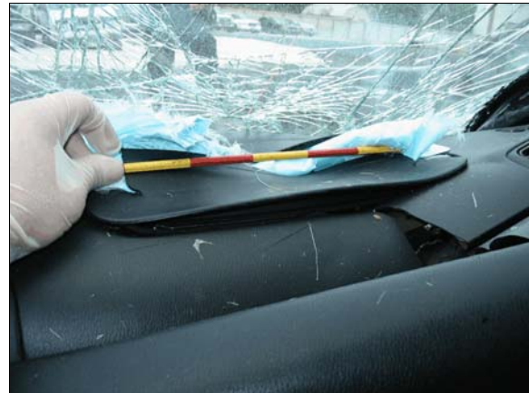
Figure 10: Front right passenger's air bag module cover flaps, the air bag was cut out by police
