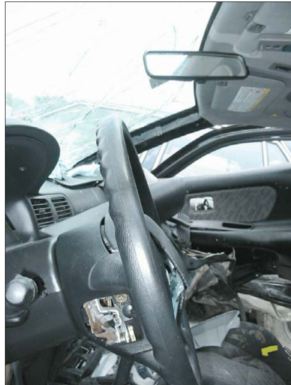
Figure 8: Steering column and steering wheel showing lack of deformation
