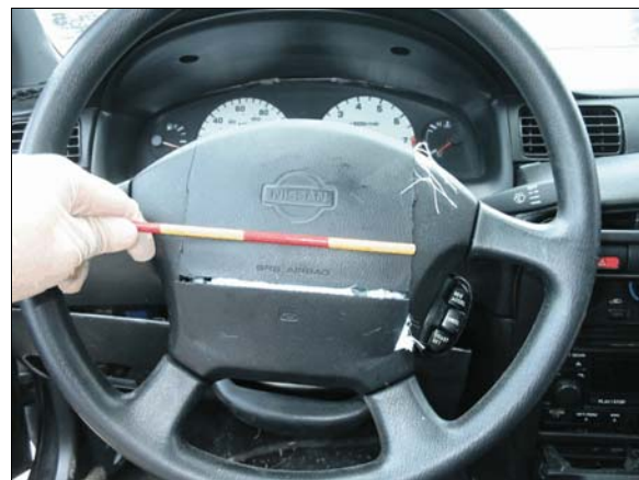
Figure 9: Driver's air bag module cover flaps, the air bag was cut out of the module by police
