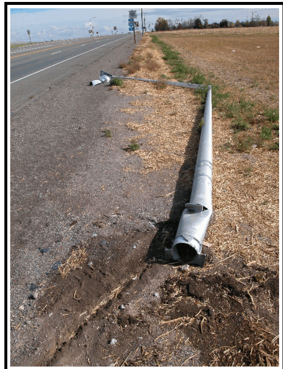
Figure 4. Damaged light pole
