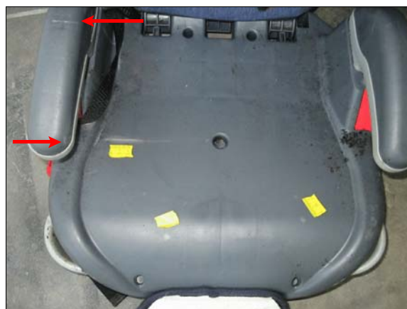
Figure 12: Yellow tape shows stress marks in plastic of case vehicle’s back left booster seat, arrows show probable occupant contact scuff on end of right arm rest and a scratch at center of arm rest
