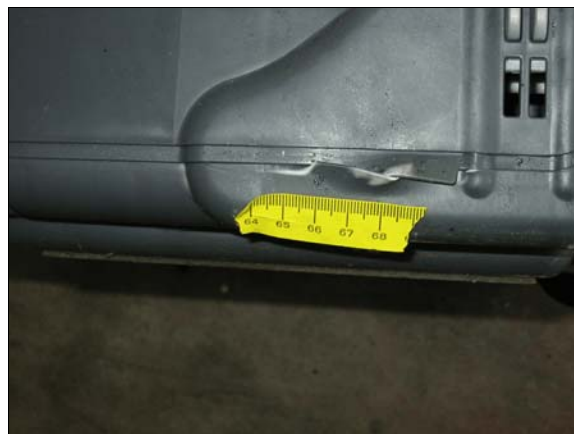
Figure 14: Displacement and damage at assembly seam on left base of case vehicle's back right booster seat
