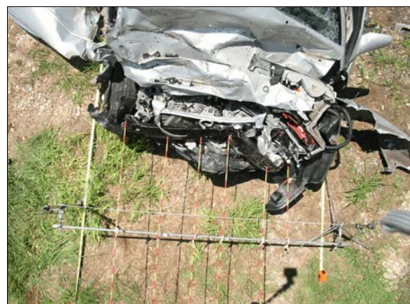
Figure 5: Top view of case vehicle's front crush, baseline is set 42 cm (16.5 in) short, final crush values reflect adjustment for this
