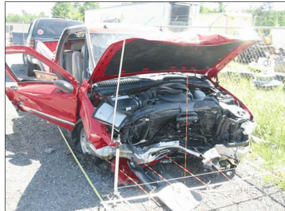
Figure 3: Overview of damage to front of GMC due to impact with the case vehicle
