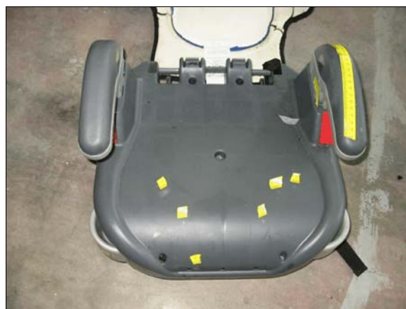
Figure 13: Case vehicle’s back right belt-positioning booster seat, yellow tape on booster seat shows small stress marks in plastic and possible occupant contact scuff and few strands of hair and cloth threads on inside of left arm rest
