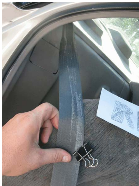
Figure 16: Load marks on case vehicle's back right safety belt
