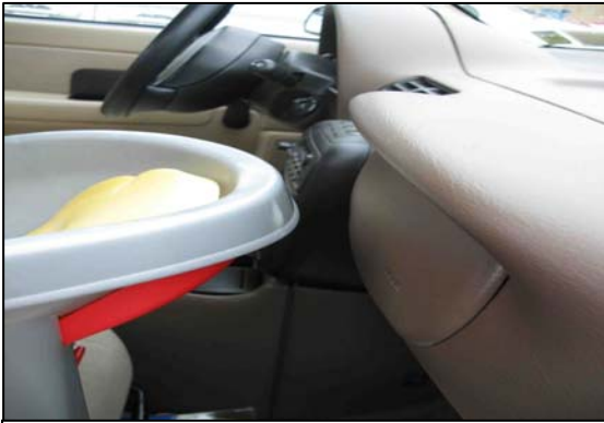
Figure 12 - Close-up of the gap between the CSS and instrument panel mid-mount cover flap.
