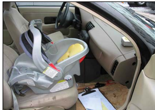
Figure 11 - View of an exemplar CSS in exemplar Saturn and distance from the air bag cover flap to the CSS.
