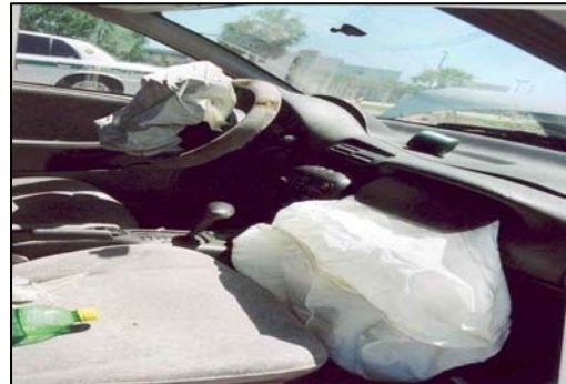
Figure 8 - Deployed frontal air bags in the Saturn.
