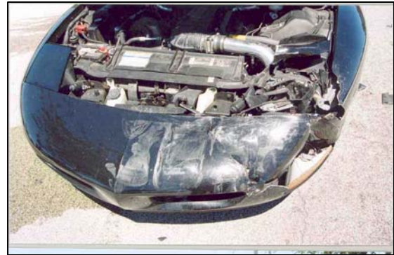
Figure 6 - Damage to front of the Pontiac.
